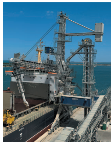
The SL1500 (1,500tph) is one of NEUERO's latest shiploaders equipped with its KIKO® system.
