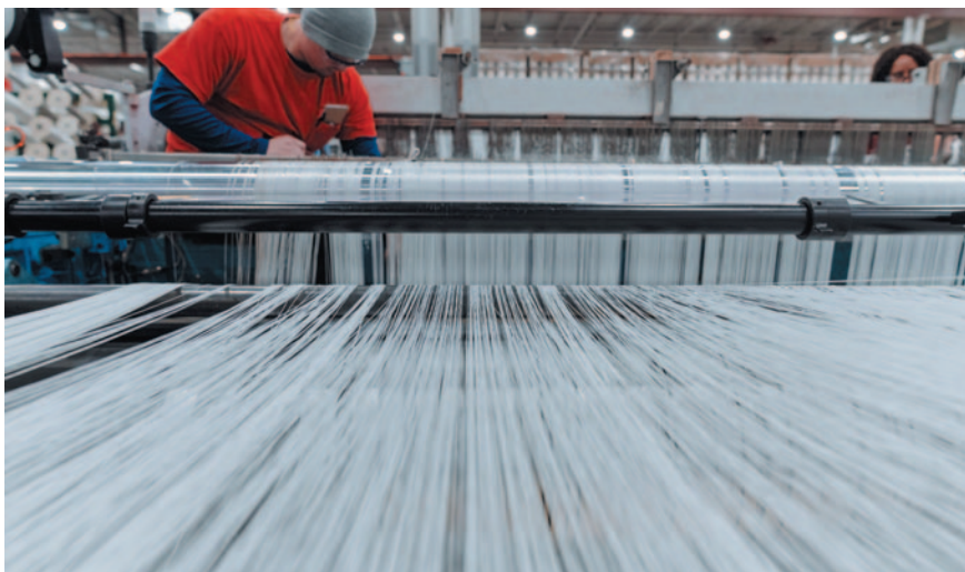
Special weave patterns using super-strong synthetic strands like Fenner Dunlop's X Series range are the best way to combat rip, tear and impact problems.
