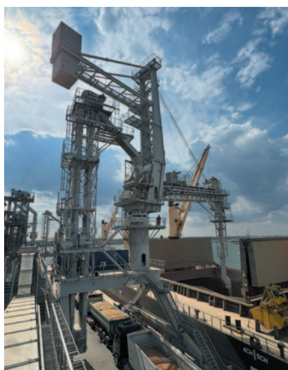
The SL1500 (1,500tph) is one of NEUERO's latest shiploaders equipped with its KIKO® system.
