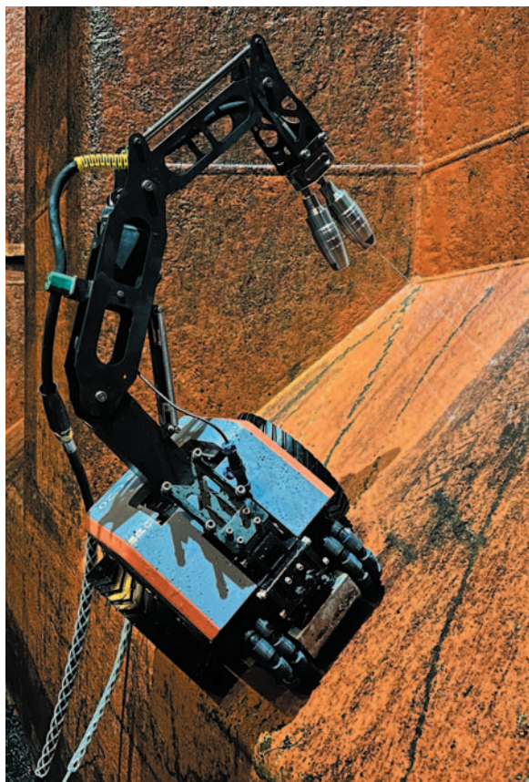
RobotPlusPlus' crawler robot can navigate angles of up to 120 degrees.
