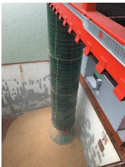
Cleveland Cascades' CC767 cascade shiploader, specified for loading grain, was supplied in 2013 to Derince Port in Turkey.
