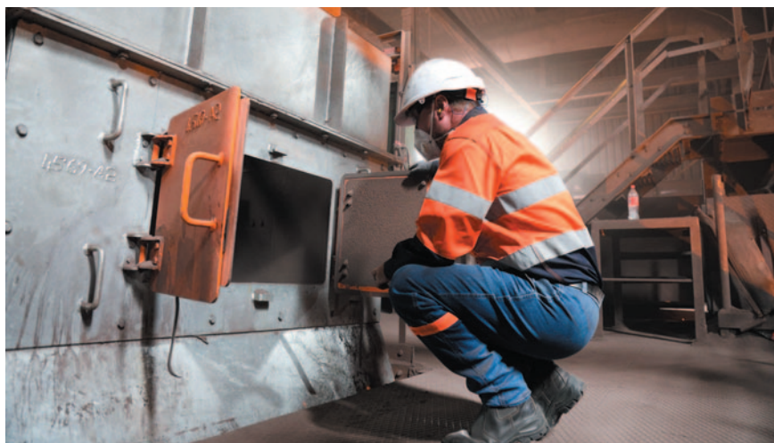
Another view of a Webba screen oversized to conveyor transfer chute installation at a steel plant, demonstrating Webba Chute Systems' ability to deliver site-specific dust-controlled transfer point solutions.
