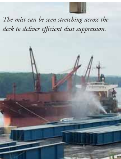
The compact size of the DustBoss allows easy positioning, and it can run continuously unattended.
