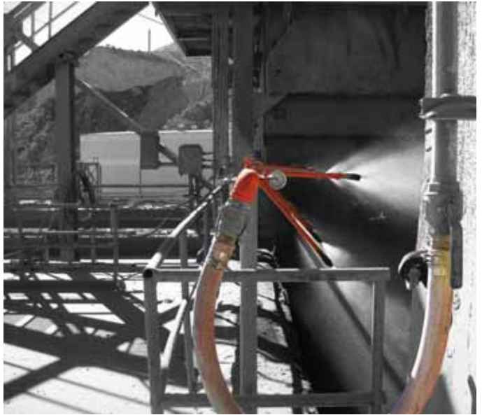
Controlled fluid sprays and specialized surfactants minimize moisture addition.
