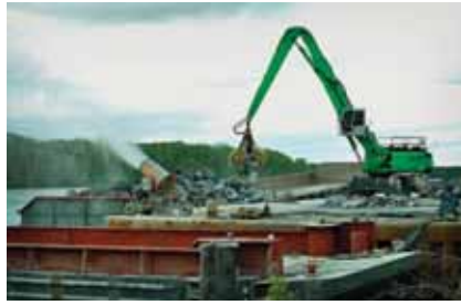
Dust suppression is directed where it is needed most in the unloading process.
