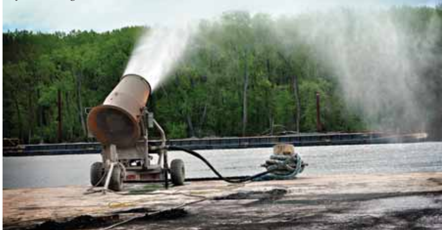
The unit features a 200-foot reach, 359° oscillation and 50° vertical adjustment angle.
