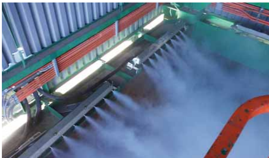
ADS™ Dry Fog uses The Raring Corp's special acoustic nozzles to fracture water into a cloud of extremely small droplets that are in the same size range as the airborne respirable dust.
