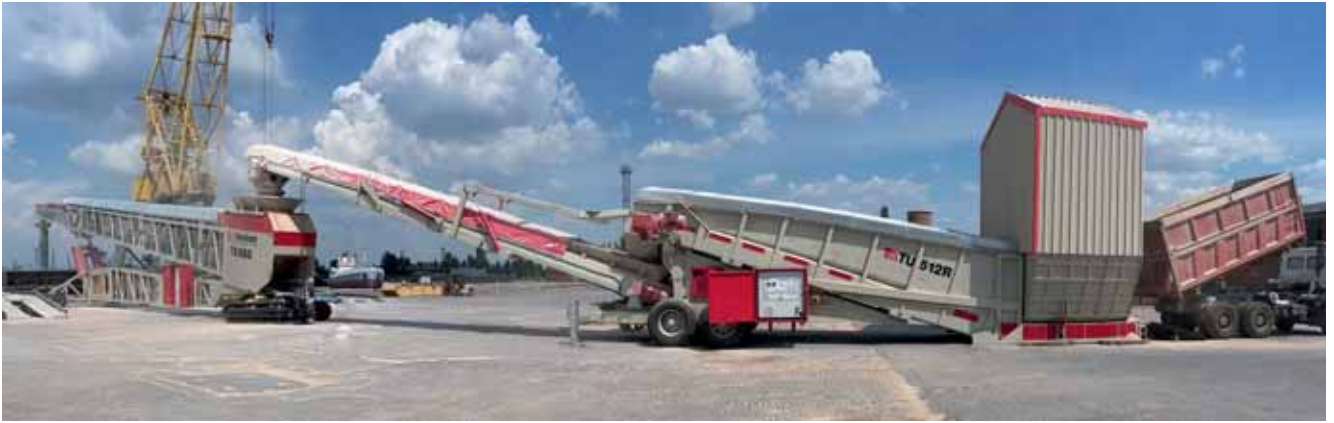
TB58 loading grain from a Titan W388-4 onto a barge in Ukraine incorporating a range of features for the grain application including dust containment enclosure and galvanized steel enclosure on the hopper incline section of the Titan unit and galvanized dust covers and telescopic chute on the TB58 and a fully enclosed transfer point between the two units
