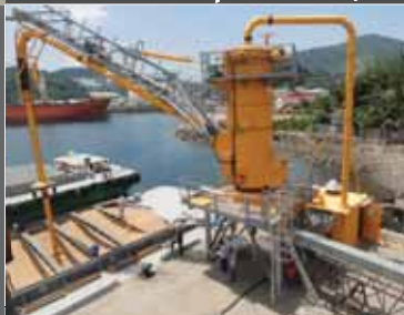
PNEUMATIC BARGE UNLOADER up to 600 t/h
