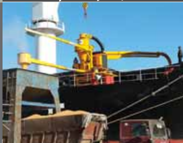
PORTABLE GRAIN PUMPS up to 270 t/h
