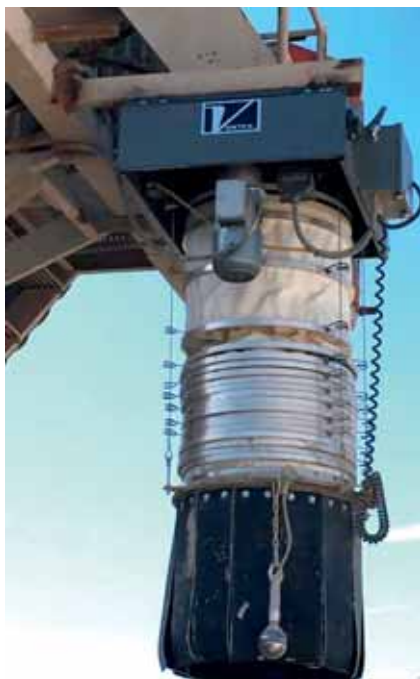
Vortex loading chutes can be designed for food-grade compliance, high temperatures, or abrasive environments.
