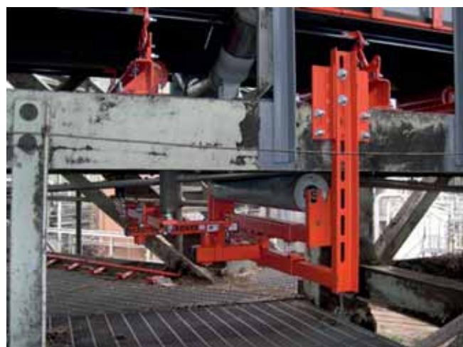
The in-line sensing roll trainer has a carrying roll on a central pivot bearing with vertical guide rolls mounted on both sides.
