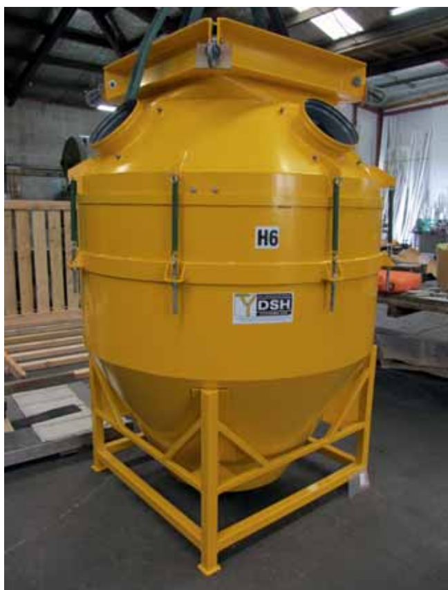
DSH unit supplied with quick release fittings for rapid inter-change of different loading devices for different applications
