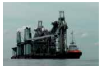
Floating loading facility Hanal ARK Shalom (self-propelled).
