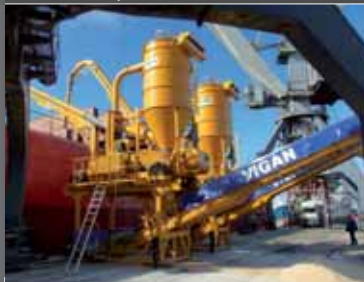
PORTABLE GRAIN PUMPS up to 270 t/h
