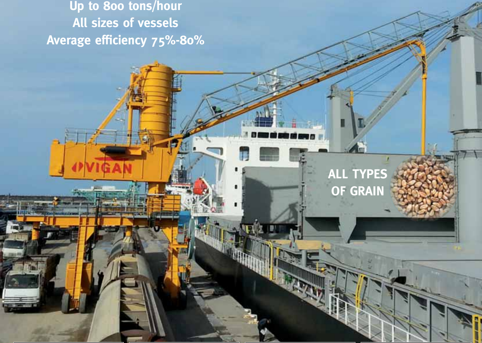
PORTABLE GRAIN PUMPS up to 270 t/h
