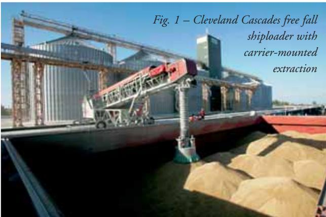
*Fig. 1 – Cleveland Cascades free fall shiploader with carrier-mounted extraction*
