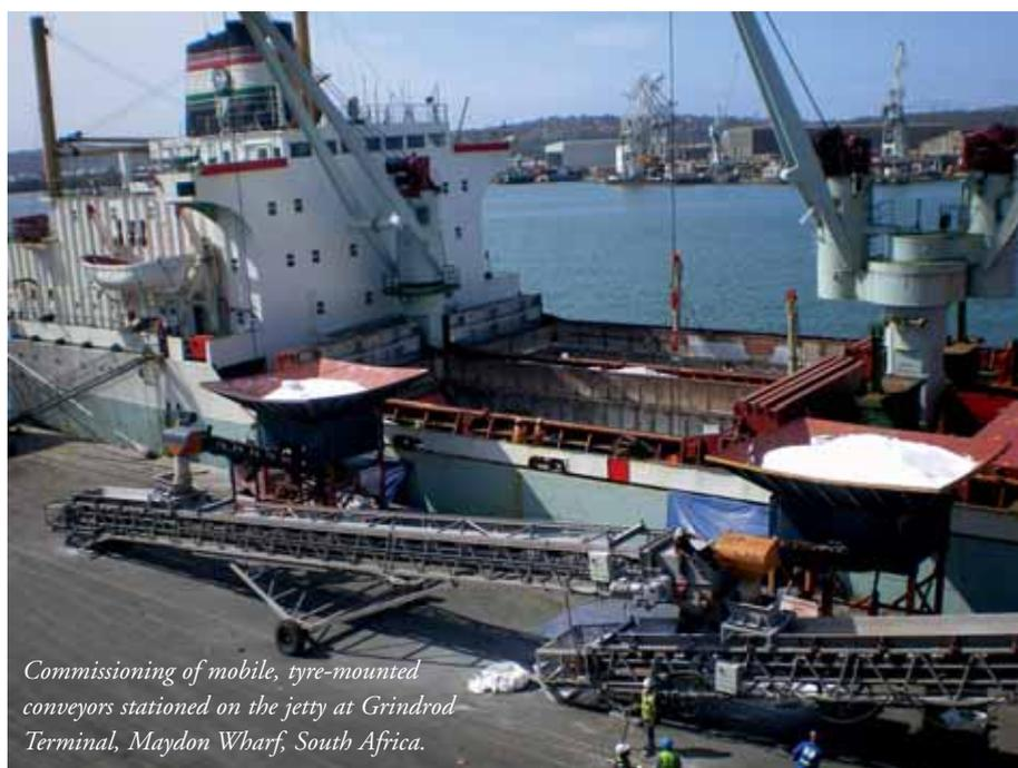
*Commissioning of mobile, tyre-mounted conveyors stationed on the jetty at Grindrod Terminal, Maydon Wharf, South Africa.*
