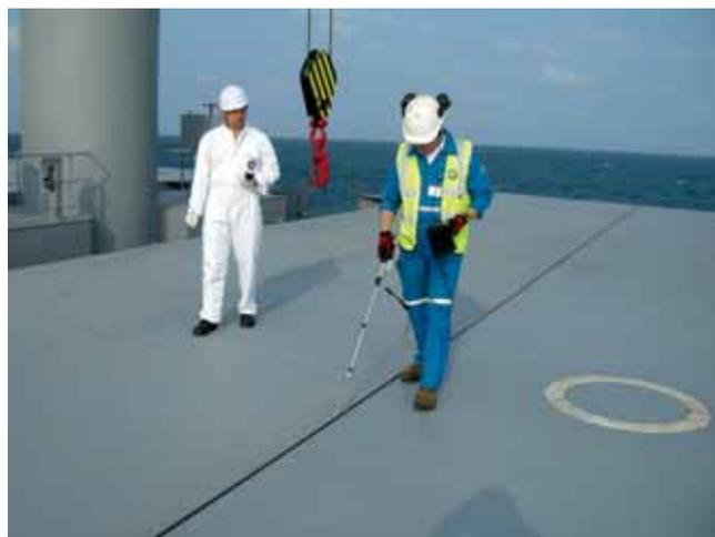
Not only does this demonstrate the benefit of this type of instruments for locating faulty rubber seals, it aids the crew to ensure proper procedure is applied in accordance with the manufacturer's recommendations for making the hatches weather tight. In addition, many ports experience sub zero
