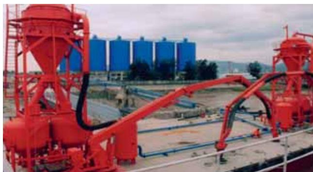
The suction arm varies in length from 12m to 35m, according to the needs of the customer.
