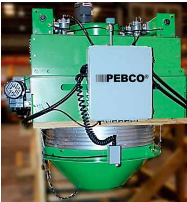
PEBCO® recently introduced the patent-pending, Self-Contained Dustless Loading System, or SCDLS. The SCDLS incorporates a dust collector integral with the loading spout. The system provides an innovative and extremely low profile design; and offers highly effective dust control for environmentally responsible loading of dry, dusty materials into trucks, railcars, ships, barges, and stockpiles.
