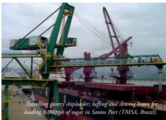
*Travelling gantry shiploader; luffing and slewing boom for loading 3,000tph of sugar in Santos Port (TMSA, Brazil).*
