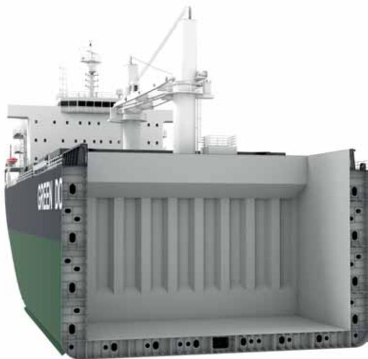
The Green Dolphin 575 was one of the projects where added resistance in waves has been evaluated in the early design phases. Here, the added resistance was calculated using SEAROS and the performance was compared to the existing SDARI Dolphin 57 design, which has similar main dimensions.
