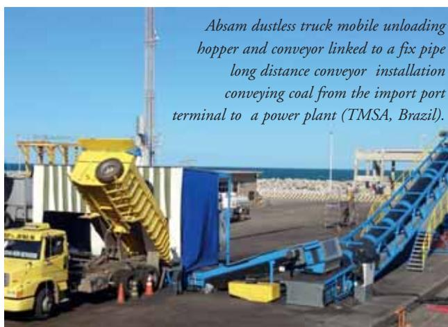
*Absam dustless truck mobile unloading hopper and conveyor linked to a fix pipe long distance conveyor installation conveying coal from the import port terminal to a power plant (TMSA, Brazil).*
