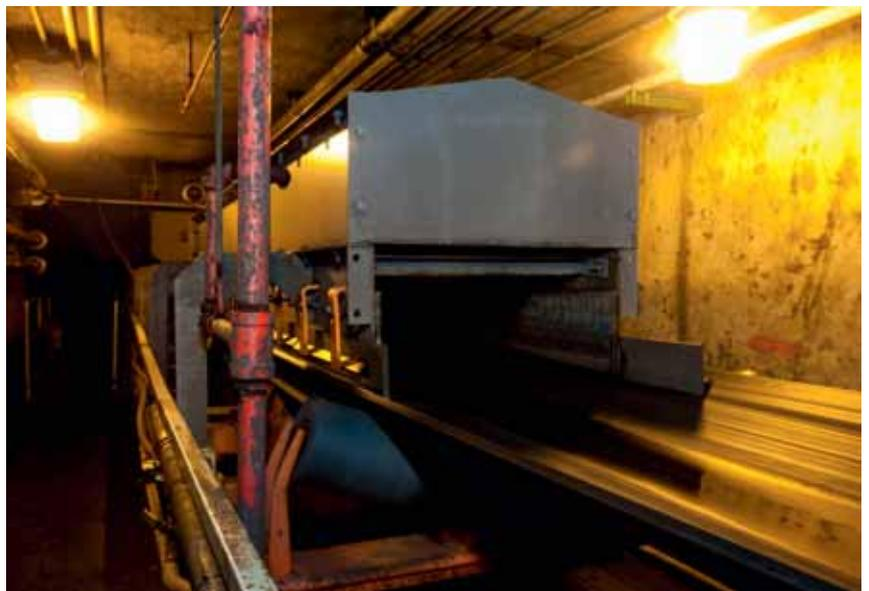
*Installed at the bottom of the loading zone skirtboard, Martin Double Apron Seal™ Skirting employs two wear surfaces on each sealing strip for twice the service life.*
