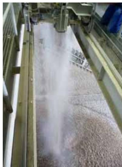
*Belt discharge from movable reversing belt with activated DUSTEX® dispersion system.*
