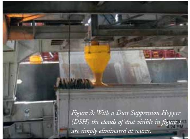
Figure 3: With a Dust Suppression Hopper (DSH) the clouds of dust visible in figure 1 are simply eliminated at source.
