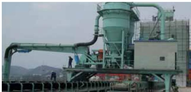
CNBM's range of pneumatic ship unloaders can be used for commodities including cement, fly ash, alumina, grain, and more. They are available in the following capacities: 20tph (tonnes per hour), 50tph, 100tph, 150tph, 200tph, 300tph, 400tph and 500tph.
