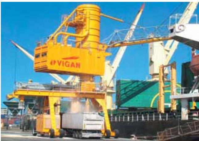
*Pneumatic unloading tower type NIV 500tph on mobile gantry, boom length: 28 metres (VIGAN).*
