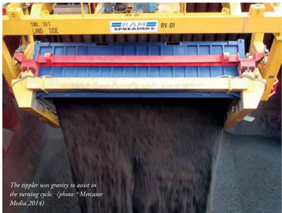
*The tippler uses gravity to assist in the turning cycle. (photo: ©Mercator Media 2014)*
