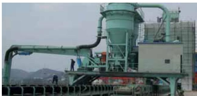
CNBM's range of pneumatic ship unloaders can be used for commodities including cement, fly ash, alumina, grain, and more. They are available in the following capacities: 20tph (tonnes per hour), 50tph, 100tph, 150tph, 200tph, 300tph, 400tph and 500tph.
