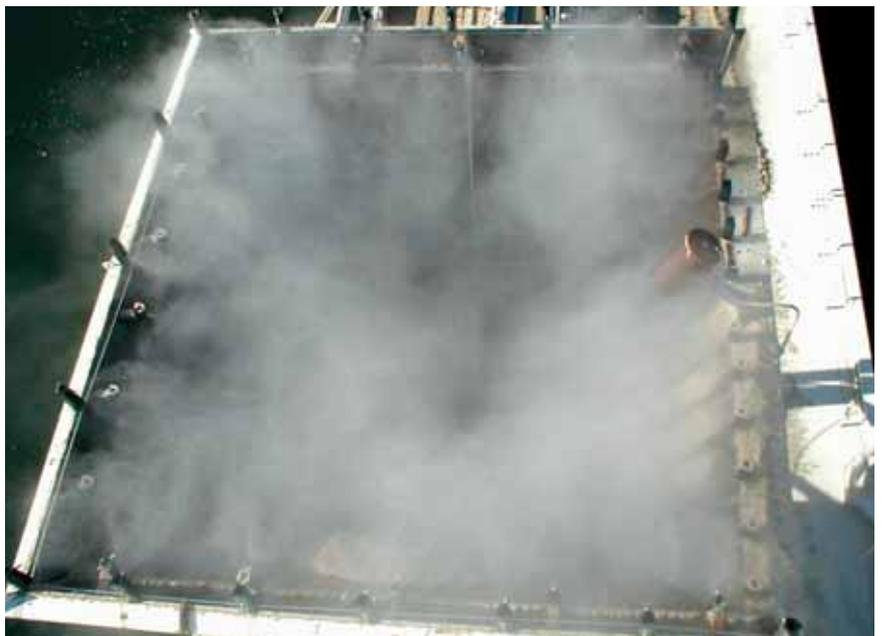
Figure 3: The high-pressure system delivers filtered water between 800 to 1,200 PSI, creating a mist-type curtain preventing the dust escaping.
