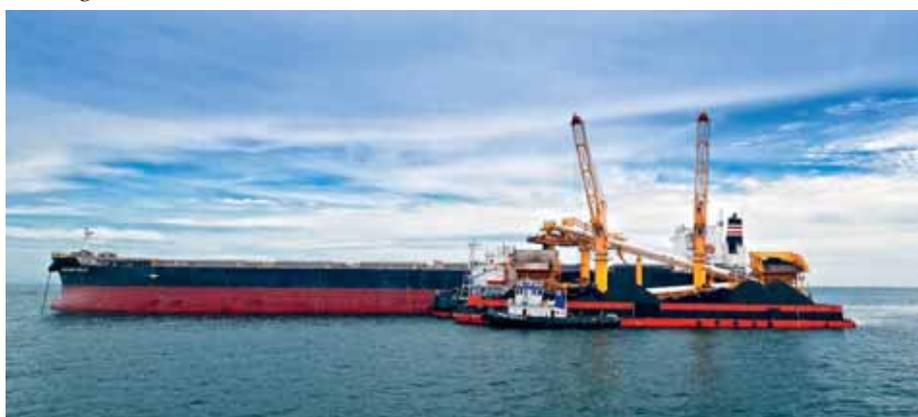
boom, the slew bearings conceived with triple roller and four equally distributed slewing motors, four-rope grab configuration, heel and trim alarm systems, thus ensuring high turnover, efficient and effortless loading/unloading from most types of vessels up to modern Capesizes.
