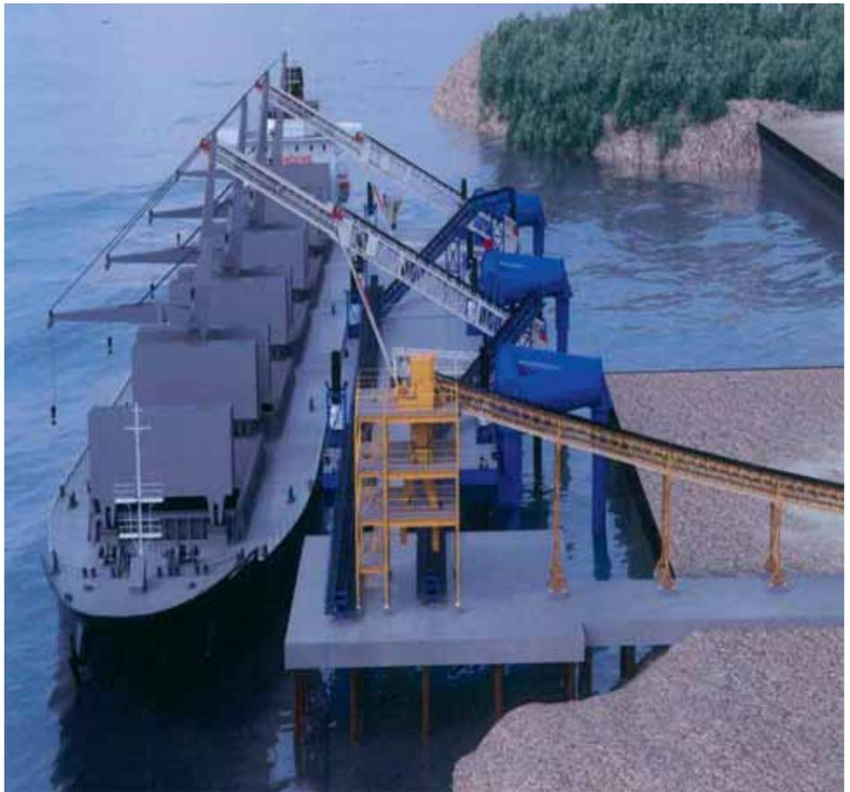
The main dimensions of the loading quay are: length 120m; width 32m; depth 3.5m; maximum deck load 10t/m<sup>2</sup>.
