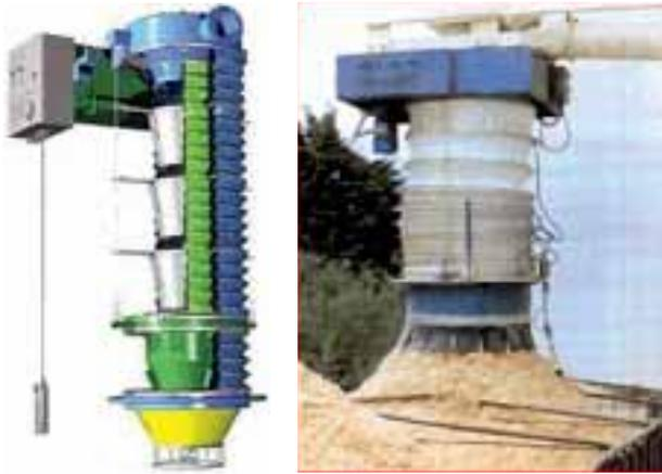
Figure 2: Conventional telescopic bellows have inherent limitations when it comes to limiting dust release.
