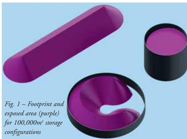
Fig. 1 – Footprint and exposed area (purple) for 100,000m³ storage configurations
