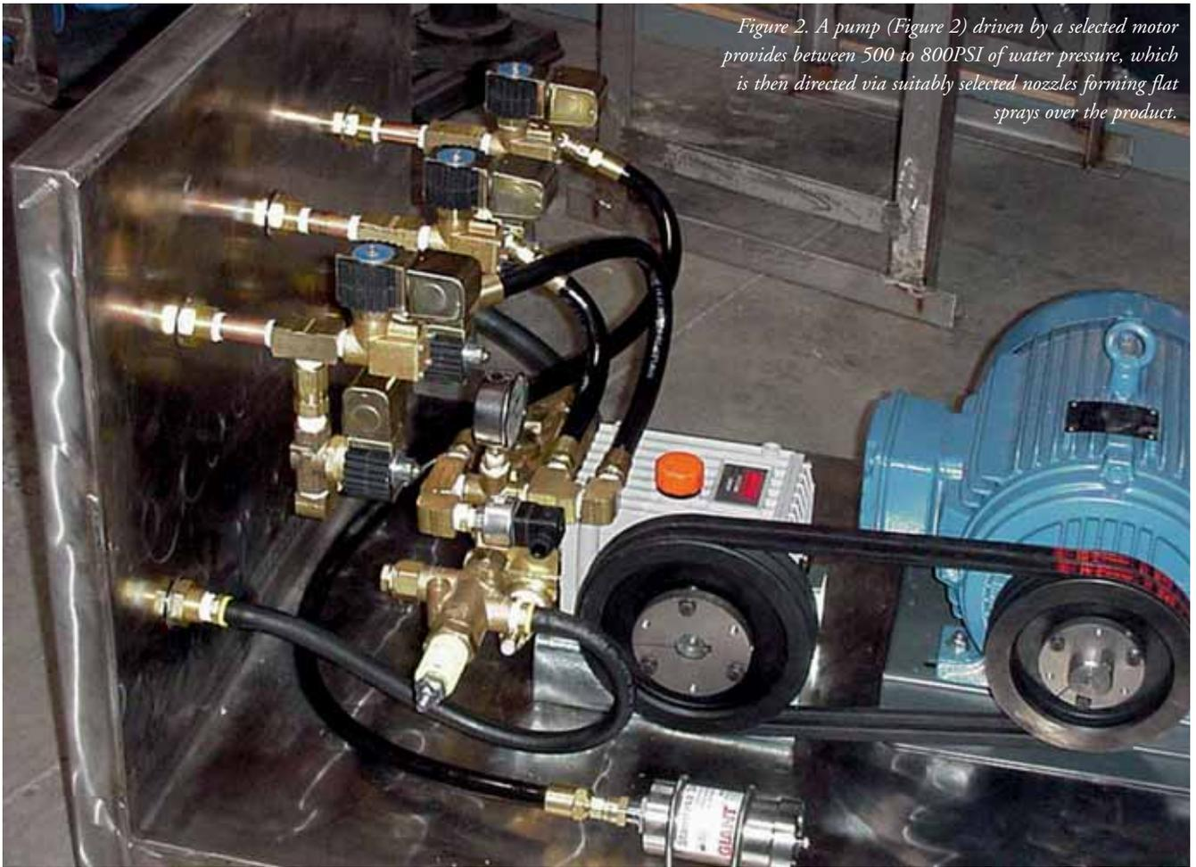
Figure 2. A pump (Figure 2) driven by a selected motor provides between 500 to 800PSI of water pressure, which is then directed via suitably selected nozzles forming flat sprays over the product.
