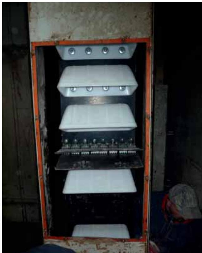
The Cobra/Transco weaving workshop has developed and produced a totally new fabric for elevator belts.
