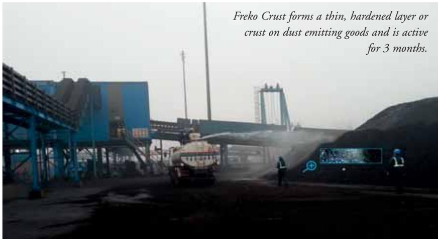
*Freko Crust forms a thin, hardened layer or crust on dust emitting goods and is active for 3 months.*
