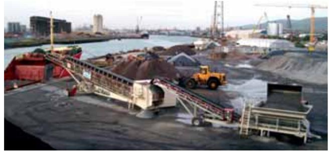
*All Travel mobile radial telescopic shiploader loading to coaster vessel being fed directly from a mobile hopper feeder (Telestack, Ireland).*
