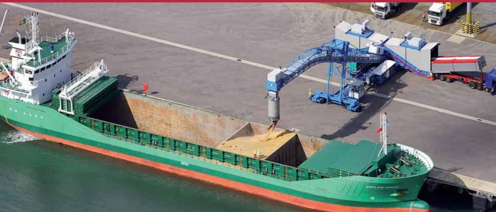
**Flexible loading direct from truck to ship**
