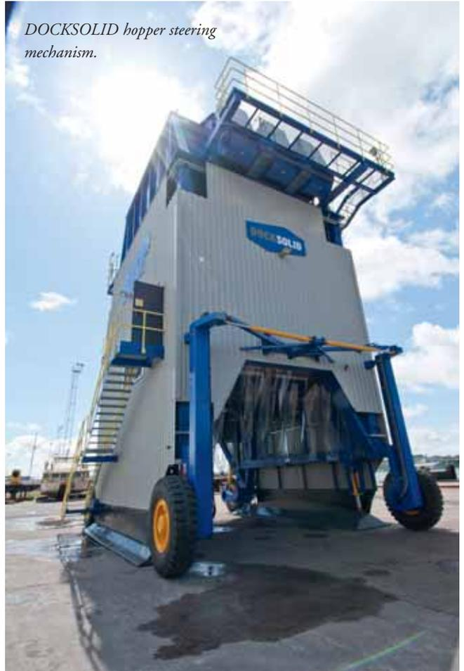
The mechanical steering design used on the DOCKSOLID hoppers is somewhat unusual; for vehicles with such a gap between wheels on the same axle, computerized steering
