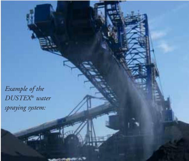
*Example of the DUSTEX® water spraying system:*
