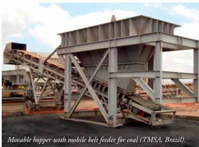
*Movable hopper with mobile belt feeder for coal (TMSA, Brazil).*
