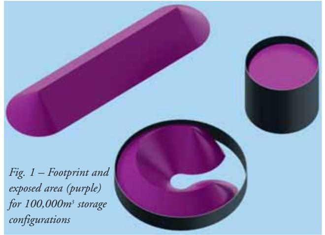
Fig. 1 – Footprint and exposed area (purple) for 100,000m<sup>3</sup> storage configurations
