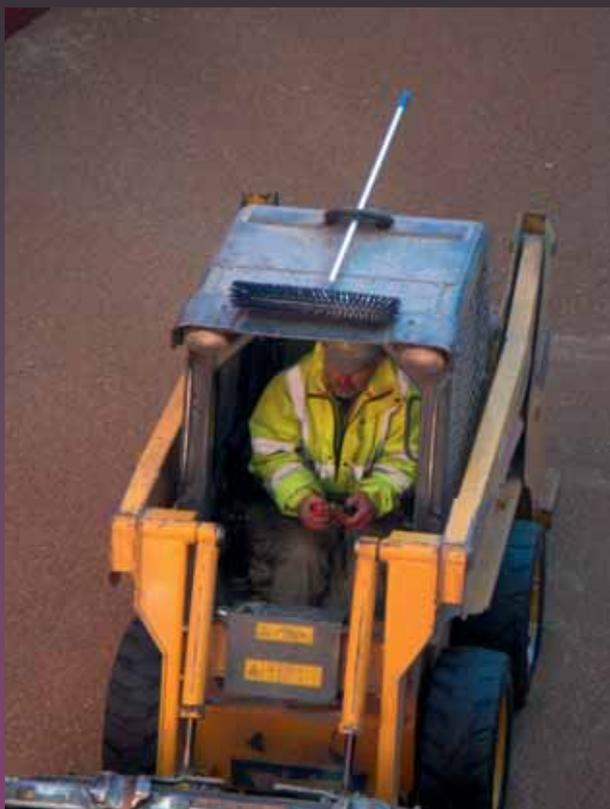
The driver of the skid steer loader type of auxiliary equipment has a control box in his hands, which allows him to guide all the movement of the horizontal and vertical telescopic suction pipes. Therefore he will be able to ensure that the suction intake nozzle is always in an optimum position ('in full heap') with large amount of grains to be seized into the pneumatic CSU.
