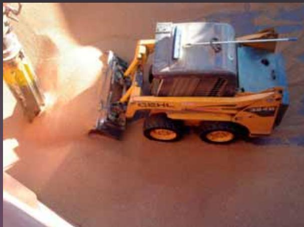
By continuous pushing of the grains towards this suction nozzle with his small size loader, the same driver will guarantee an optimum use of the pneumatic CSU handling capability.
