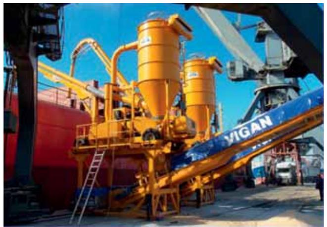
*Mobile type 200 with diesel engine, 9m front boom and transfer conveyor capacity up to 270tph (cereals) (VIGAN).*
