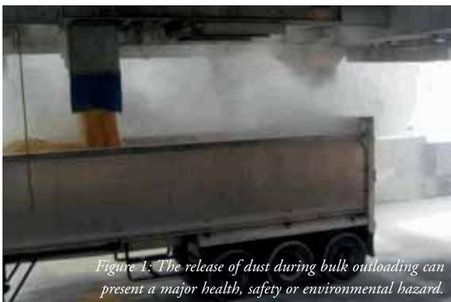
*Figure 1: The release of dust during bulk outloading can present a major health, safety or environmental hazard.*
