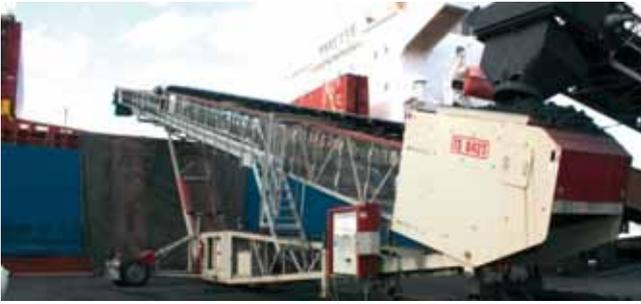
*Telestack telescopic mobile shiploader loading to Panamax vessel.*
