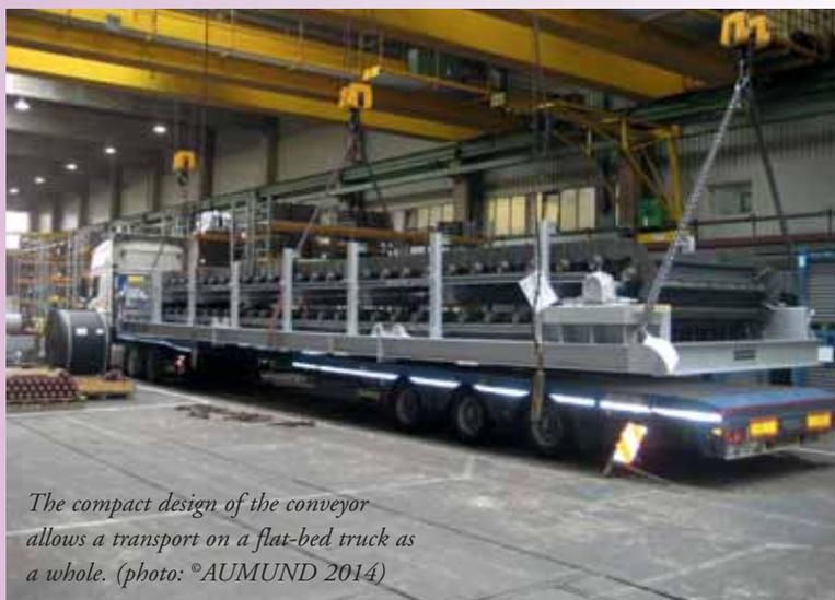
*The compact design of the conveyor allows a transport on a flat-bed truck as a whole. (photo: ©AUMUND 2014)*
