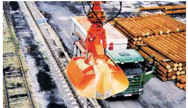
Type KZH: The enclosed construction, which protects the environment, is clearly evident in this hydraulic grab.
