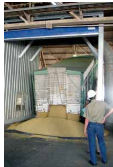
Fig. 10. Port terminal truck dumping station in Argentina at pit of Fig.6, and after the DustMaster system with confined cabin.
