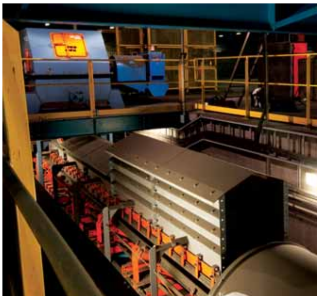
The extended height settling zone from Martin Engineering is designed to decrease air velocity and increase settling time.
