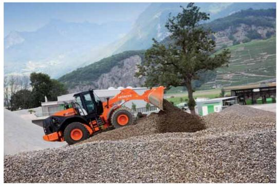
For operation in dust-filled environments, the ZW-5 wheel loader can be equipped with an optional wide-pitch fin radiator to prevent clogging. Another useful feature for quick routine maintenance is the automatic reversible cooling fan, which allows for easy cleaning of the radiator with its one-minute automatic reverse rotation every 30 operating minutes.
