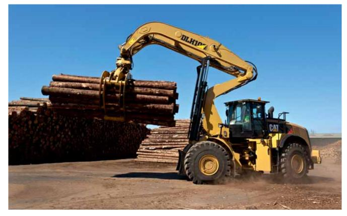
Caterpillar and Demlone have partnered to create a high-lift log handler based on the Cat<sup>®</sup> 980 wheel loader and a log grapple and front designed and built by Demlone. The new log handler complements the extensive line of Cat Forestry machines and enables Cat dealers to offer a total solution for material handling needs around the wood yard and in port situations. The Demlone DLH100k Log Handler will be commercially available this month (September) this year.
