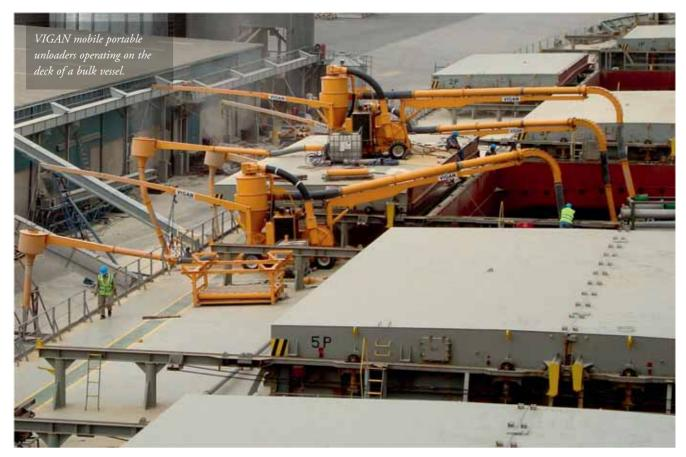
Since 1967, VIGAN Engineering S.A. has been designing and manufacturing portable pneumatic unloaders, commonly called 'mobiles' or 'grain pumps':
