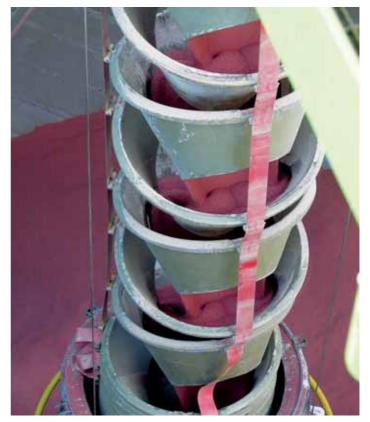
**Case Study 1:** Potash – ThyssenKrupp, Germany The Cleveland Cascades cascade system was developed with the safe handling of potash in mind. This close-up shows the unique cascading of the material throughout the length of the chute, which minimizes the build-up of corrosive dust particles.
