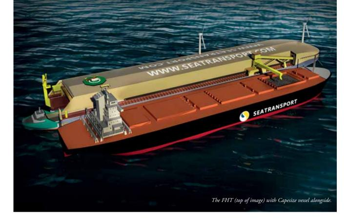
thrusters to keep the combination of the FHT and export vessel out of a beam sea wave vector, to avoid a synchronous rolling situation.
