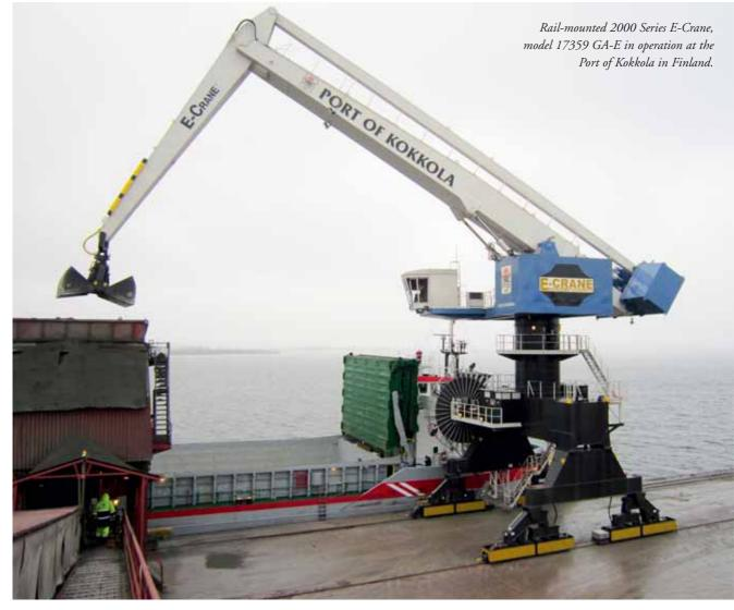
Last month (see p103 of the August 2012 issue of *Dry Cargo International*), we discussed how an E-Crane on a floating terminal can be an economical solution for expanding your port infrastructure. This month, we'll be focusing on how mobile E-Cranes are a practical solution for any mobile needs at your facility. E-Cranes can be installed on either low or high gantry portal on rails, or on crawlers.
