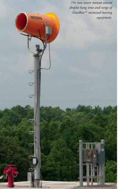
can deliver a focused mist to the areas where dust is created," commented DCT general manager Laura Stiverson. "This allows the DustBoss<sup>™</sup> units to concentrate virtually their entire output directly to the source of the problem." Designed to withstand wind loads of at least 100mph (miles per hour), the towers are constructed of carbon steel pipe, hot dip galvanized to resist corrosion.
