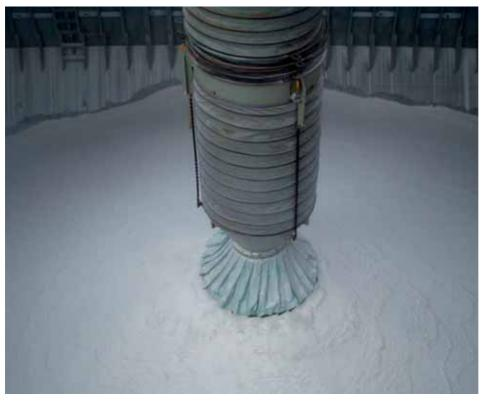
**Case Study 2:** Alumina – Voest Alpine, Australia. In terms of dust emission control, alumina is one of the most problematic materials to handle. With particle sizes of less than 75µm, airborne dust can be a risk to both operator health and the wider environment. Note that the entire Cleveland Cascade chute is clearly visible in the confined space of the ship's hold, and dust is minimized, despite loading rates of up to 1,500tph.
