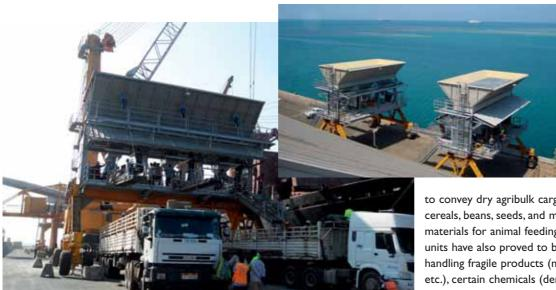
mobile hoppers/ bagging lines, like for the grain port terminal of Djibouti (see pictures left). Originally, all VIGAN equipment was designed
