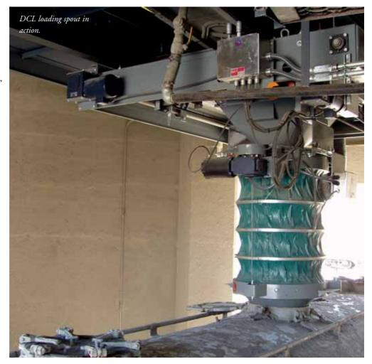
horsepower silo aeration reclaim system for fine products; pedestal-style articulating loading arms to include automatic inline tracking; telescopic air-slide ship loading boom; and nonmechanical deadfall spout discharge for dust control of fine products in shiploading
