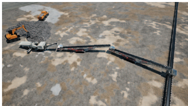
Two TCL 2031 conveyors working as a link conveyor onto a reclaiming line from a Primary Jaw crusher.
