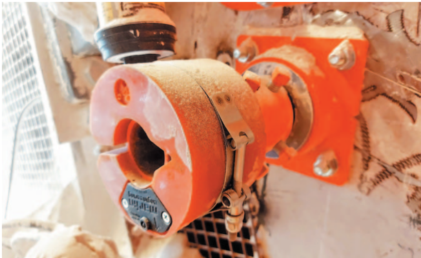
Copyright © Martin Engineering 2025. Martin's N2 Position Indicator provides data on the condition and performance of each belt cleaner.
