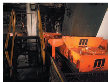
Figure 8: a tail box helps prevent backflow of spillage and dust at the rear of the chute.
