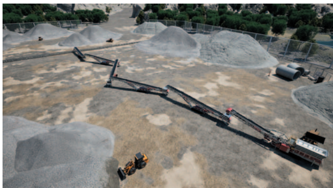
Five TCL 2031 conveyors working as a link conveyor with the HF 24T heavy duty hopper feeder in reclaiming / mining applications.
