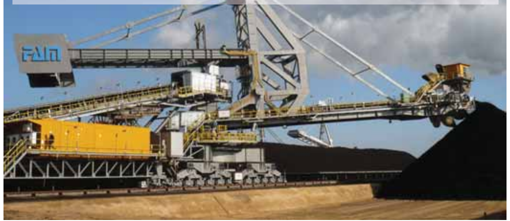
Figure 1: FAM stacker-reclaimer STR11000/7500.42 with a reversible boom conveyor is used in a coal-fired power plant in Germany for both stacking and reclaiming. As a stacker, the machine receives the material for stockpiling via a tripper car (11,000tph), and as a reclaimer, it unloads the stockpile using a bucketwheel (7,500tph).
