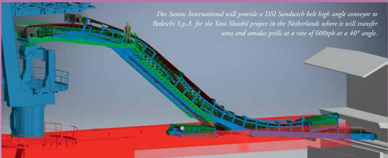
*Dos Santos International will provide a DSI Sandwich belt high angle conveyor to Bedeschi S.p.A. for the Yara Sluiskil project in the Netherlands where it will transfer urea and amidas prills at a rate of 600tph at a 40° angle.*
