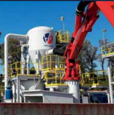
**Road mobile ship unloaders up to 250 tons per hour**
