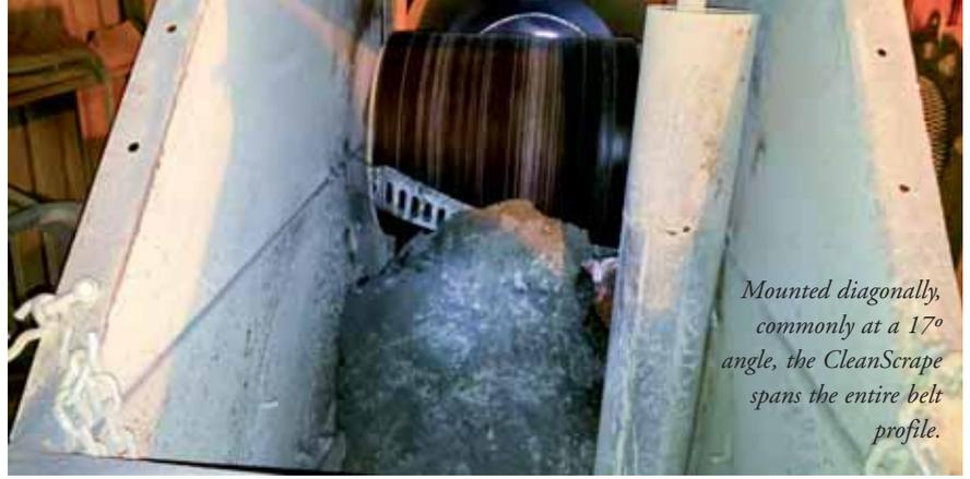
*Mounted diagonally, commonly at a 17° angle, the CleanScrape spans the entire belt profile.*
