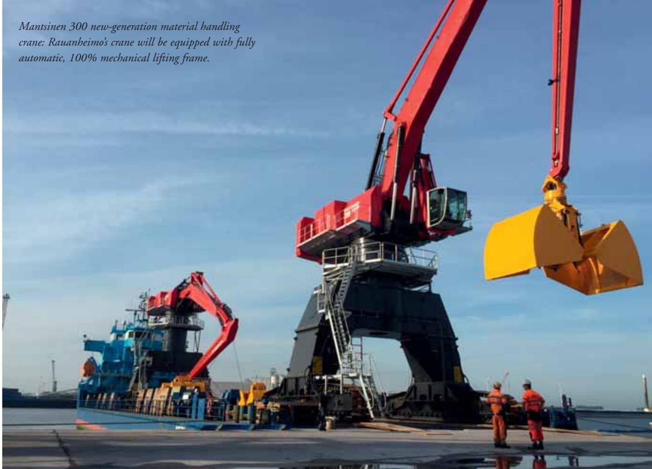
terminal and loading quay added pressure for cargo delivery during shiploading. Therefore, Rauanheimo acquired a new generation material handling crane — a Mantsinen 300 equipped with fully automatic, 100% mechanical lifting frame and, in co-operation with a Finnish manufacturer, has developed a new type of transportation platform, the 'PULPHAULER'. This development breaks with traditional methods, and makes it possible to double the efficiency of moving cargo from the terminal to the quay.
