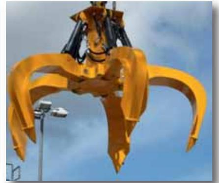
unique hydraulic self lubrication system uses the grab's working pressure to drive the self-lubrication grease pump. The system pressurizes grease up to 250 bar and injects grease to all main bearing and cylinder bearings —15 bearings in total.
