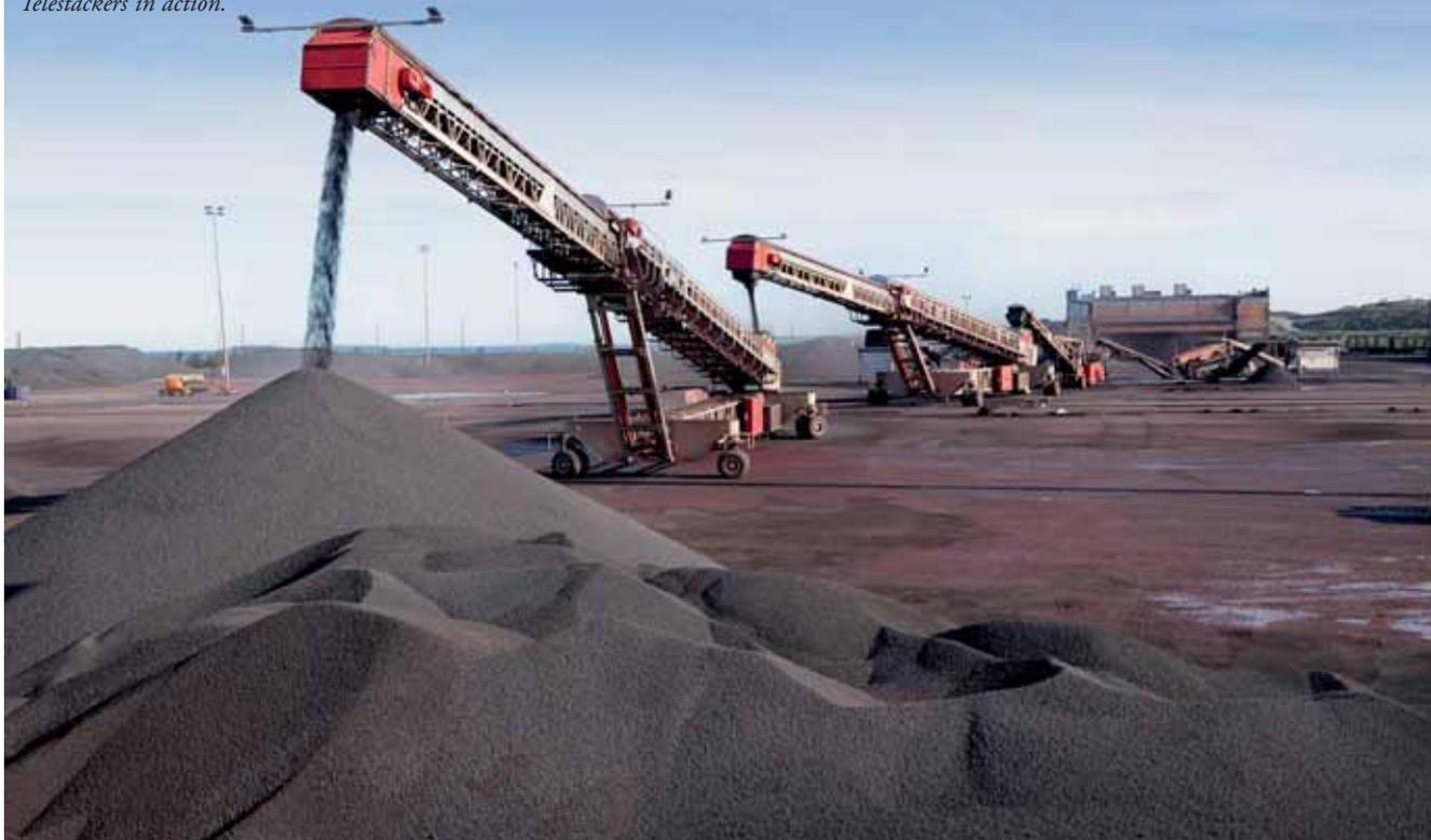
equipped with two hoppers, one for feeding with a wheel loader and one with dump trucks. These units can also be connected together to move the material from the train unloading facility directly under the crane, avoiding the processing phase. The conveyor system is also suitable for different type of solid bulk cargo.
