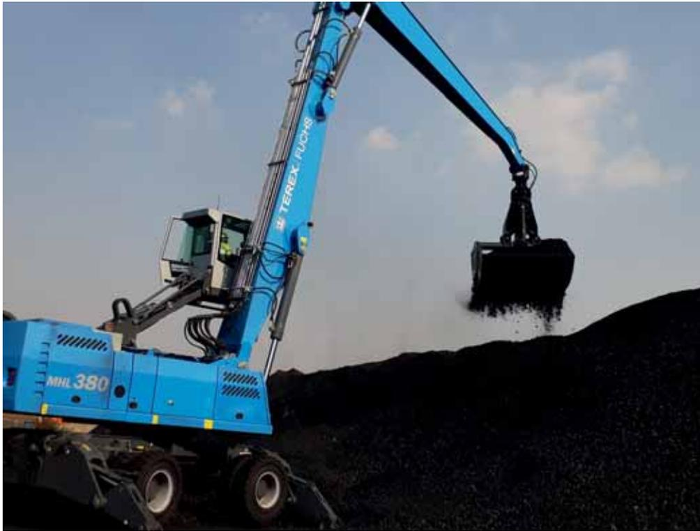
features are helping Makoya's machine operators to increase loading efficiency and boost machine uptime. The MHL 380 handler's spacious cab hydraulically adjusts to a 6.2m maximum eye level, allowing the operator to easily see over the sides of the rail wagons even when fully laden.
