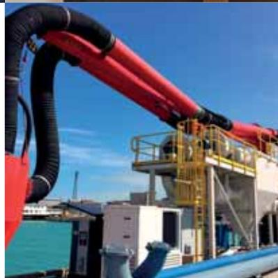
**Bulk handling equipment for dusty abrasive materials like cement, fly ash, alumina**
