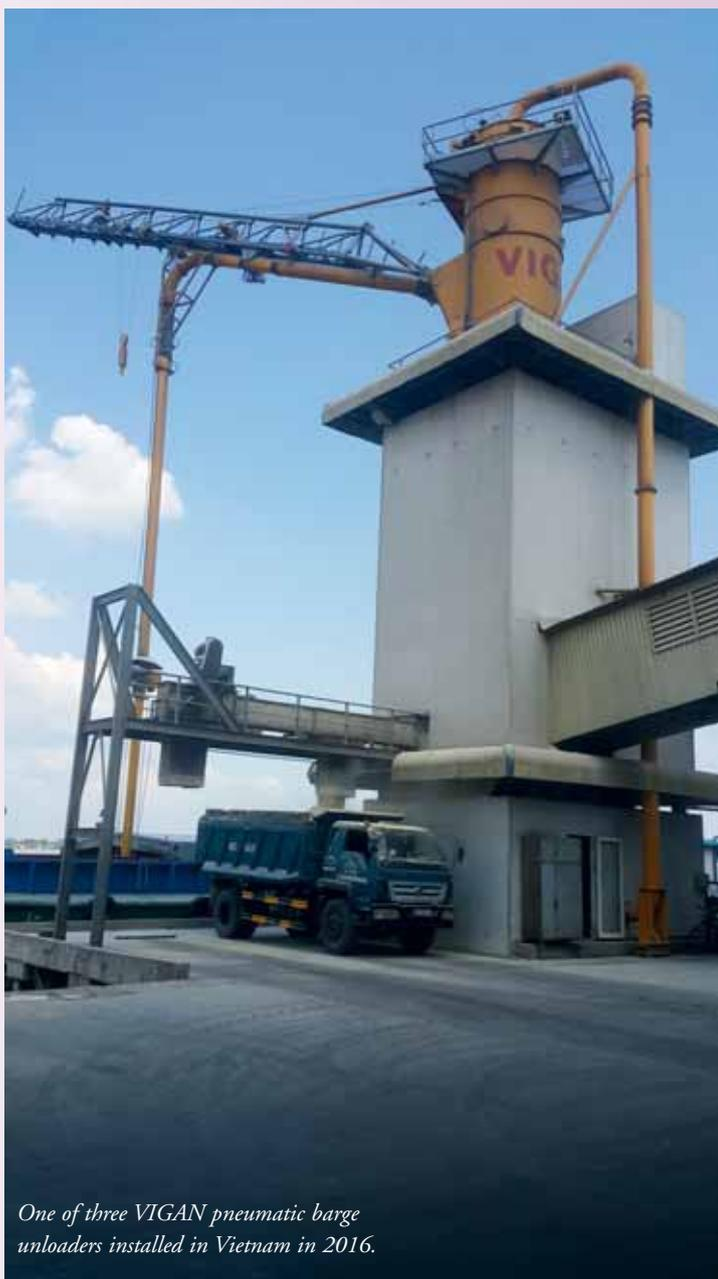
*One of three VIGAN pneumatic barge unloaders installed in Vietnam in 2016.*
