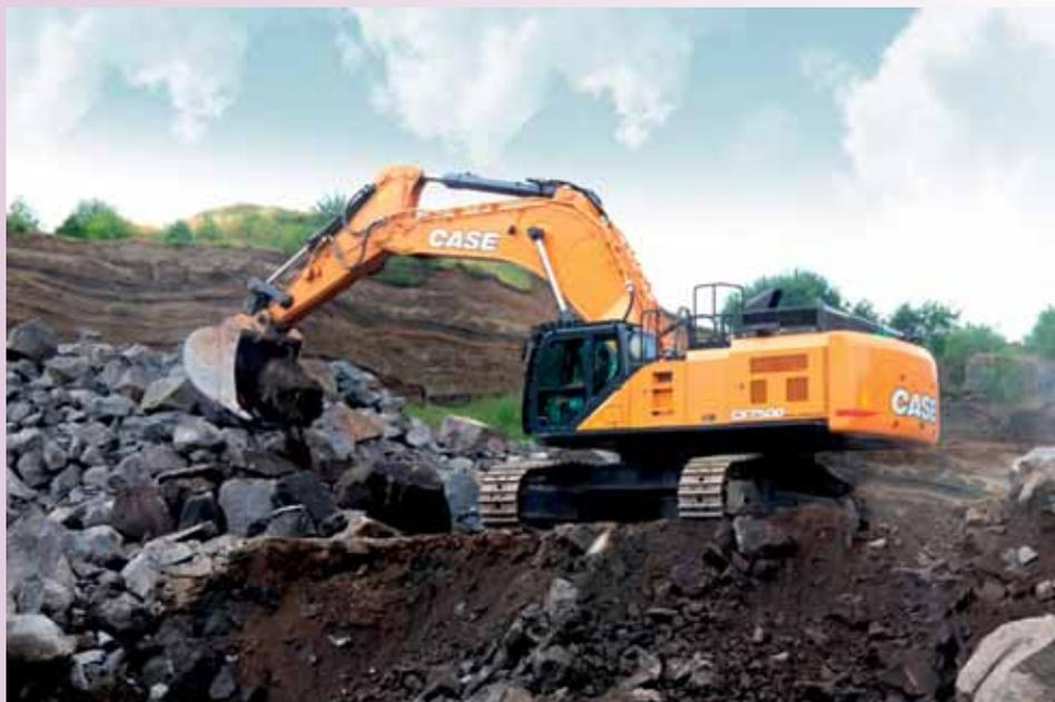
for greater power and productivity, and arm and bucket cylinders are larger to help improve performance. And the machine can be operated in one of three operating modes — Automatic, Heavy and Speed Priority — to provide the optimal and most efficient use of hydraulic and engine power.
