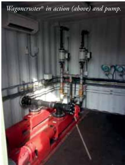
In a special foam generator, using two litres of dbd FO 312® and 98 litres of water, a staggering 5,000 litres of foam is created.
