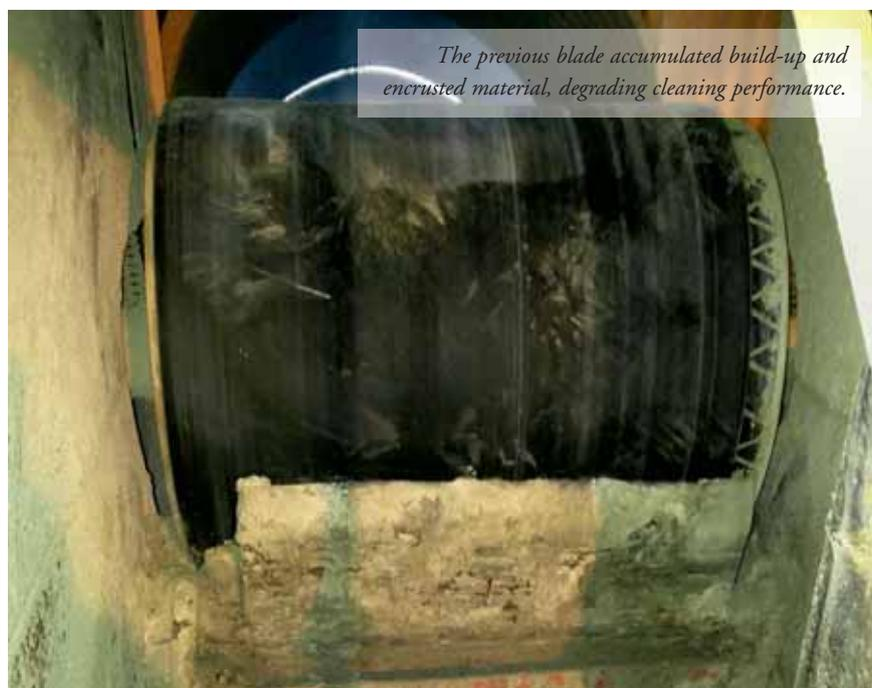
*The previous blade accumulated build-up and encrusted material, degrading cleaning performance.*
