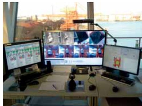
loading. It helps reduce human interaction to the process to a bare minimum and hence makes it not only possible to control the entire loading process from a remote location but also to provide an unprecedented level of automation, enabling one operator to feed several ship or train loaders from multiple, blending capable sources easily from a central control room.
