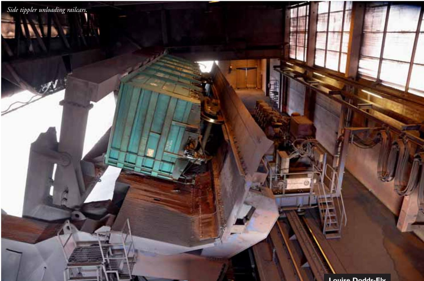
*Side tippler unloading railcars.*
