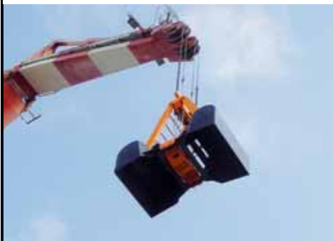
Mechanical four rope clamshell bucket
