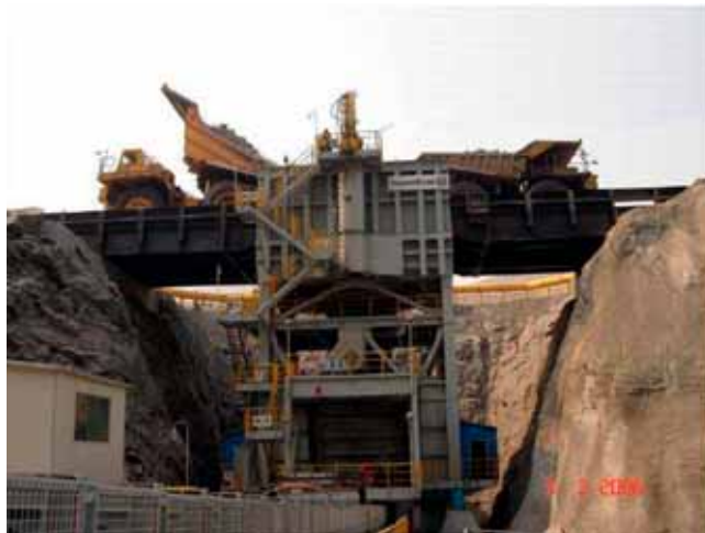
A semi-mobile crusher plant for iron ore, similar to that for Shougang Hierro Peru, just put into commercial operation at Tangang Mine, China.
