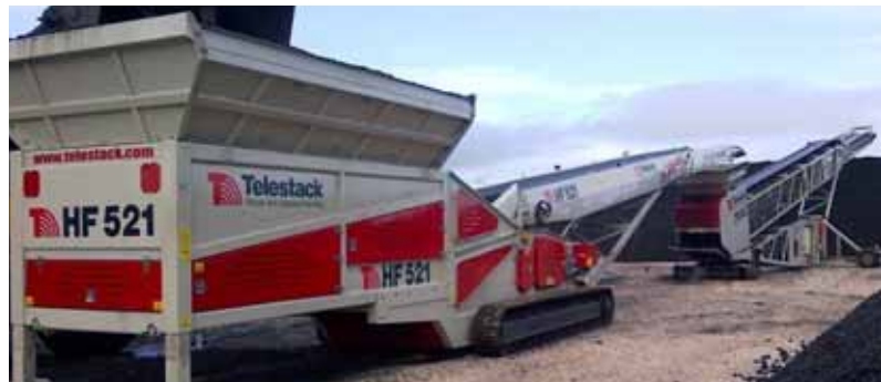
Hopper Feeder & Radial Telescopic reclaiming/ stockpiling coal in stockyard of powerplant
