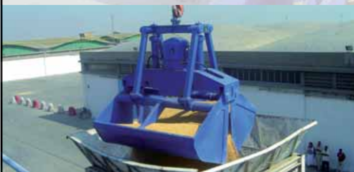
Electro hydraulic clamshell bucket
