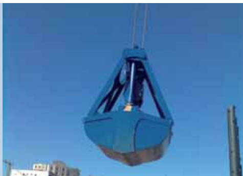
Mechanical one rope clamshell bucket
