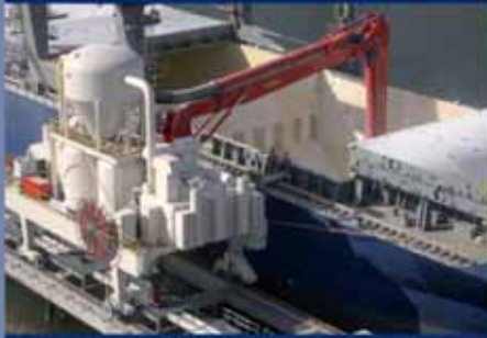
Rail Mounted Ship Unloader
