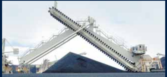
Portal Scraper Reclaimer with Twin-Boom
