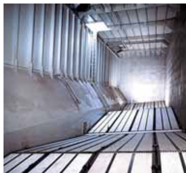
The revolutionary IBAU HAMBURG Tunnel concept: Midship tunnel with the IBAU Pump and aeration panels.
