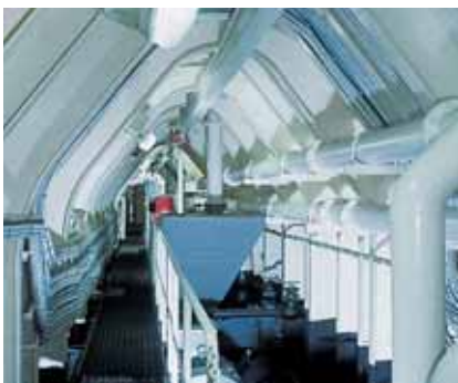
The revolutionary IBAU HAMBURG Tunnel concept: Midship tunnel with the IBAU Pump and aeration panels.
