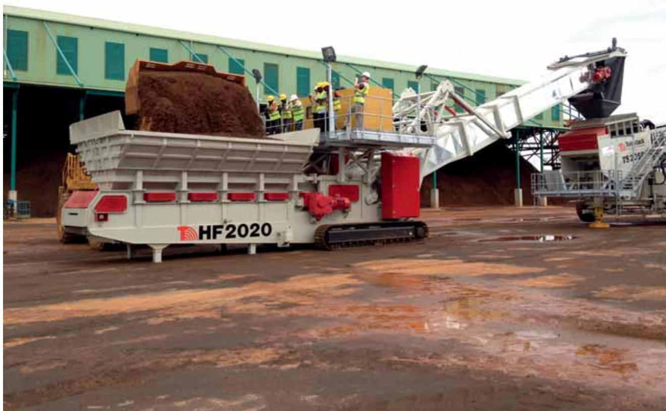
Figure 4: heavy duty hopper feeder transfer point with auto sampling system.
