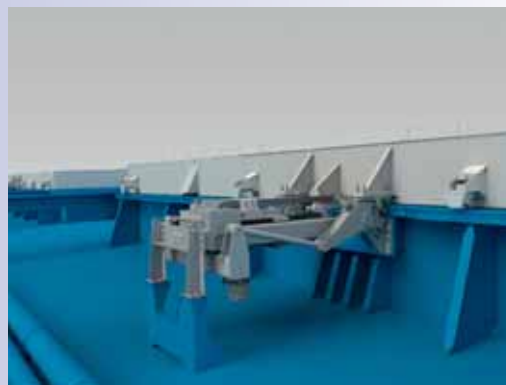
MacGregor's innovative MacRack technology — each hatch cover panel is operated by an electrically-driven MacRack unit, which both lifts the panel up and rolls it to its open, stowed position in 2.5 minutes.
