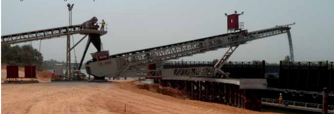
Fig 8: TS 1550 radial telescopic shiploader loading the 8,000dwt barges at 1,500tph.
