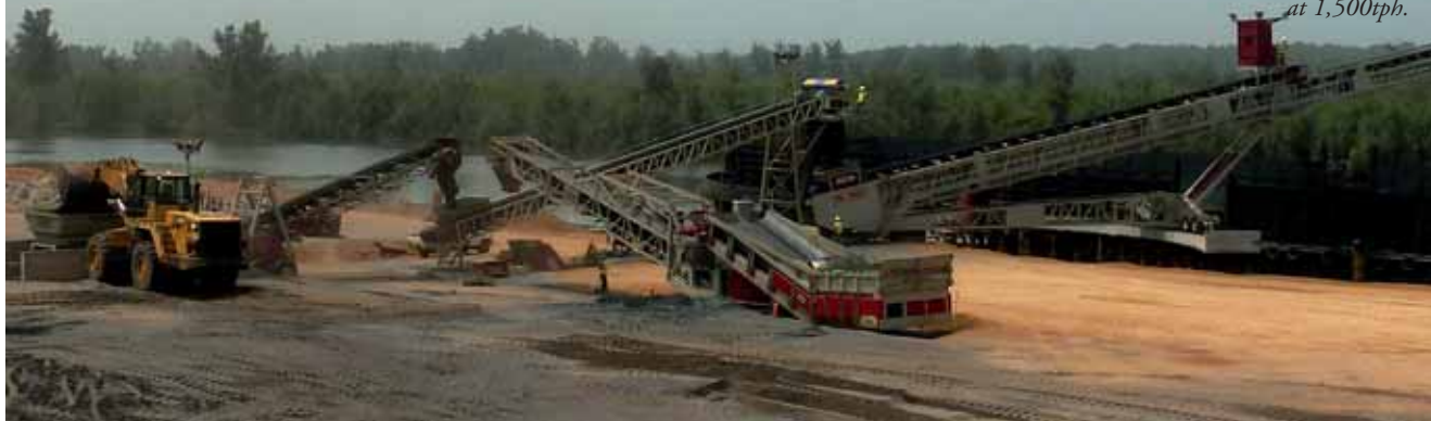
Fig 8: TS 1550 radial telescopic shiploader loading the 8,000dwt barges at 1,500tph.
