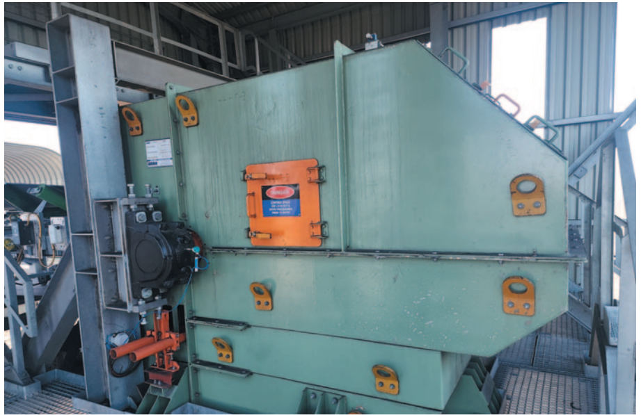
A Weba Chute Systems conveyor transfer chute in operation at a Mpumalanga mine, efficiently transferring thermal coal with minimal spillage and wear.
