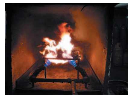
Class 4A involves a more severe fire test according to EN 12881-1 method A, C or D.
