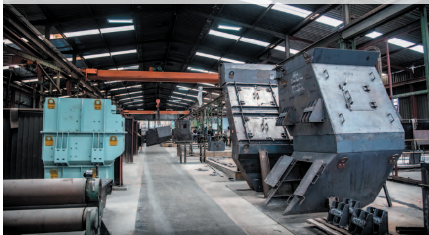
Custom-engineered transfer chutes are being manufactured at Weba Chute Systems' Wadeville factory in Germiston, ready for delivery to mining customers.
