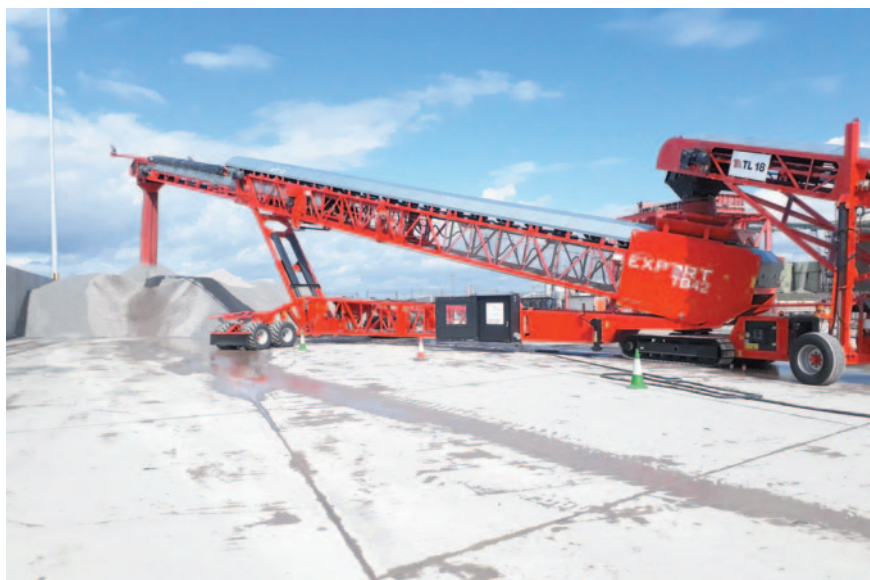
Multi-purpose Telestack system used for shiploading and unloading (stockpiling).
