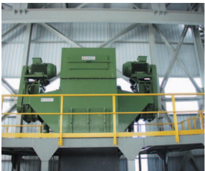
Image 2 & 3: MDG ESPLV head stations equipped with double drive.
