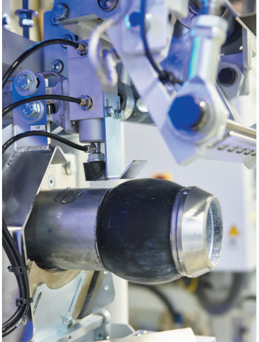
Specialized inflatable filling spouts seal the bag to the spout throughout the filling process. This translates to no dust escaping through the valve and, when filling is complete, the bag is removed from the spout, and the valve is welded shut by an ultrasonic sealing unit.
