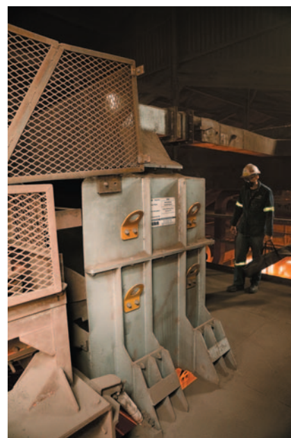
This Weba screen oversize-to-conveyor chute installation demonstrates how advanced flow control and sealing methods reduce dust, spillage and excessive wear at a steel plant.
