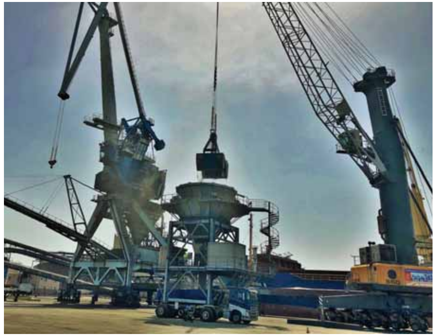
First clinker unloading at Sete port for Cem'in'Eu, directly onto truck and using a dust-free hopper to limit dust contamination.
