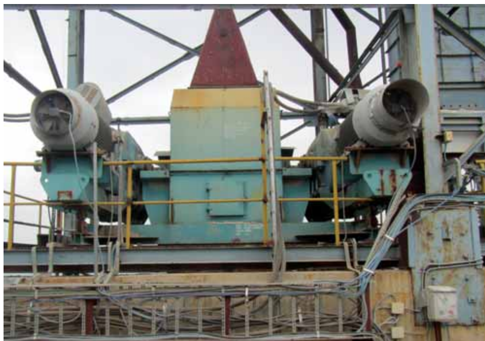
Deep pan conveyor feeding mill hopper.
