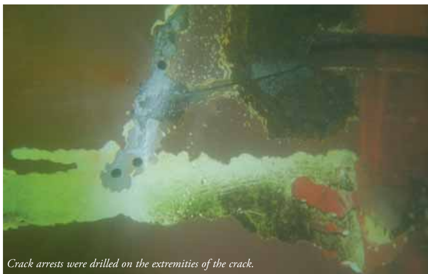
Branching crack on rudder of ro/ro ship.
