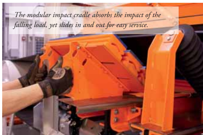
Slider cradles support the belt to prevent spillage from belt sag and eliminate material entrapment points.
