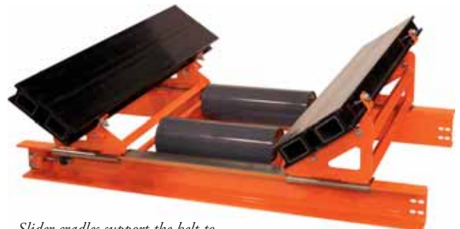
Slider cradles support the belt to prevent spillage from belt sag and eliminate material entrapment points.
