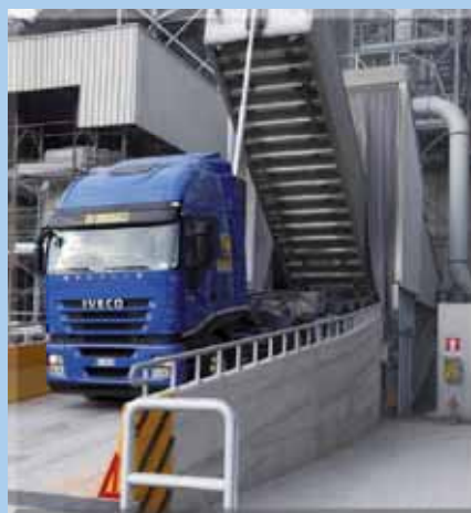
"TIREX" - Receiver from trucks and feeder for several bulk materials
