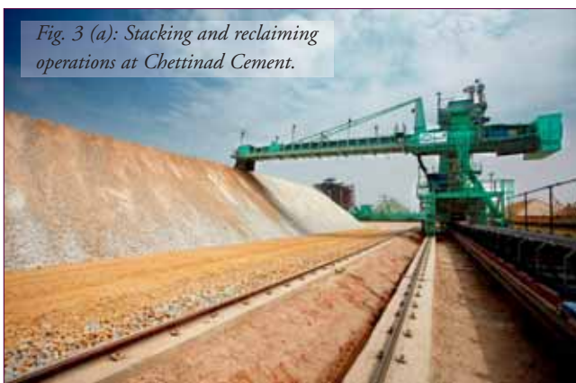
Fig. 3 (b): Stacking and reclaiming operations at Chettinad Cement.
