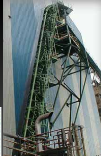
DSI Snake Sandwich High Angle Conveyor elevating coal at a 75° angle for a steel plant in Northern Spain.
