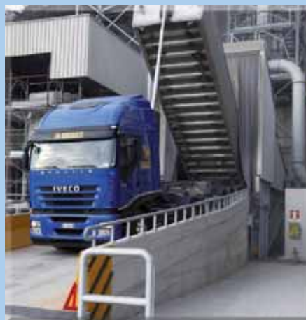
"TIREX" Receiver from trucks and feeder for several bulk materials
