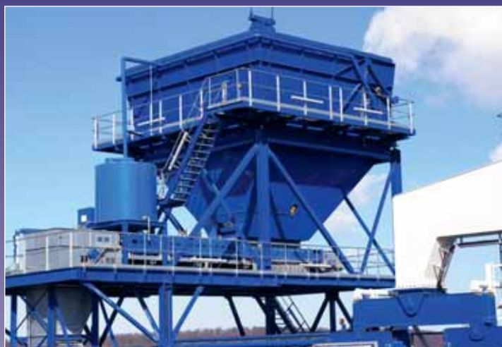
Hopper cars for ship unloading
