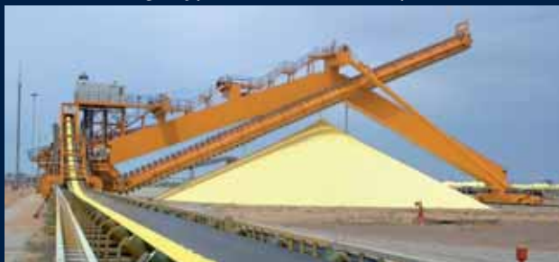
Combined Stacker / Reclaimer, sulphur prills
