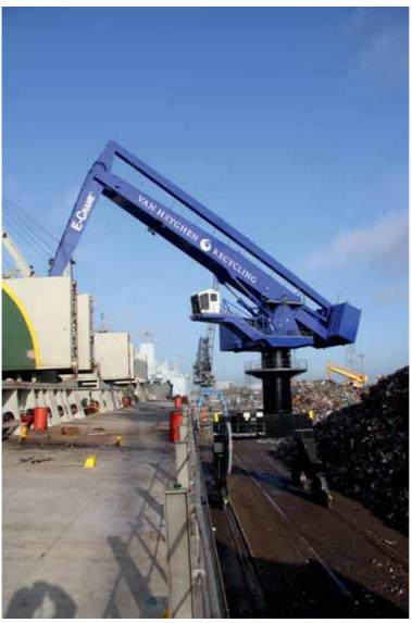
Handymax vessels, loading rates of 3,500 to 4,000 tonnes per shift are no exception for the E-Crane.
