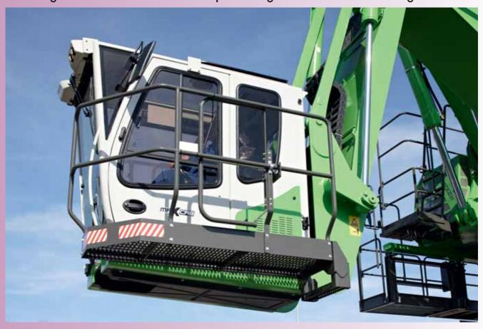
The SENNEBOGEN maXcab industrial cab is used wherever challenging material handling tasks are carried out. To make the working environment even more ergonomic and safe for drivers, SENNEBOGEN offers an optimized industrial cab model in the special equipment range to replace the maXcab comfort cab. The industrial cab offers an outstanding feeling of space and optimal overview thanks to the tilted vertical front windscreen with armoured glass and a bigger field of vision.
