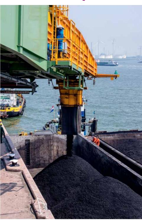
In June 2012 iSAM AG finished commissioning its first shiploader for barges and seagoing vessels at Europees Massagoed-Overslagbedrijf (EMO) BV in Europort Rotterdam, Netherlands. In line with other equipment at the largest transshipment terminal for iron ore and coal in Western Europe, the new shiploader has a maximum throughput capacity of 6,000tph (tonnes per hour) for iron ore and will be fully automated for man-less operations by the end of 2012. Even at lower rates,
