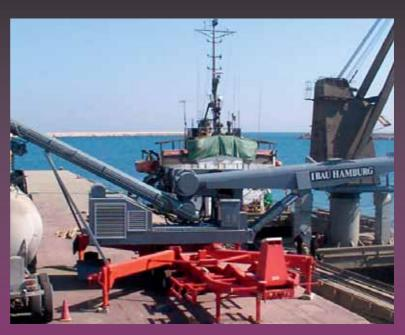
expectations, with the lowest energy consumption and the highest flexibility. The ship-unloader integrates the latest modular design, which allows for customized functions and features and specifically engineered downstream cement transport systems to the final storage.
