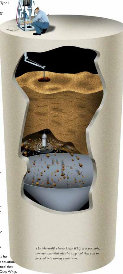
Abrasion-resistant steel chain is best suited for most applications, with non-sparking brass chain for combustible materials. Urethane flails can also be employed to protect lined
