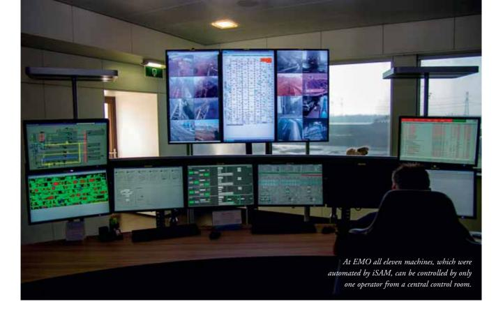
the coherent solutions for stacker reclaimers and grab unloaders. iSAM's product line now offers unique automation and optimization solutions for man-less operations in every business handling dry bulk materials like import/export terminals or mines. At EMO all eleven machines, which were automated
