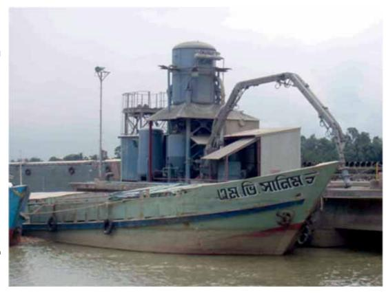
industrial duty 'vacuum cleaners'. A hydraulically manoeuvered suction boom digs into the cement in the barge hold and a suction pipe sucks out the cement to a pair of dense phase transporters on a wharf-parked
