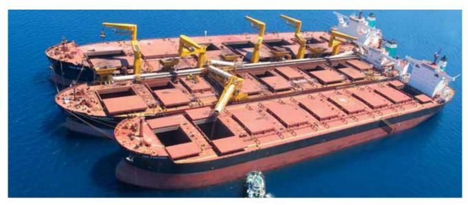
In the year 2012 two transshippers on which cargo handling systems have been supplied by Bedeschi have been commissioned — *Ore Fabrica* and *Royal Sesa*. One is for discharging iron ore from ocean going vessels and other one is for loading iron into them.
