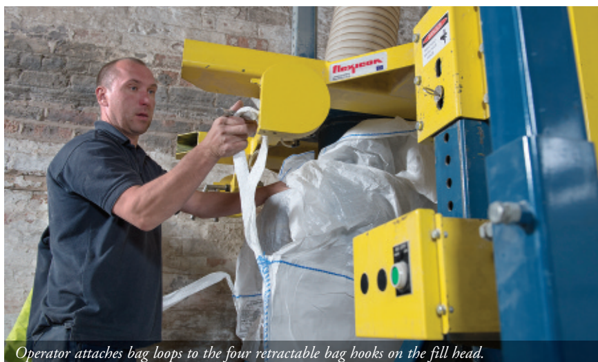
Bag spout is connected before malt is transferred from a silo through a horizontal flexible screw conveyor and downspouting into the bulk bag filler inlet.
