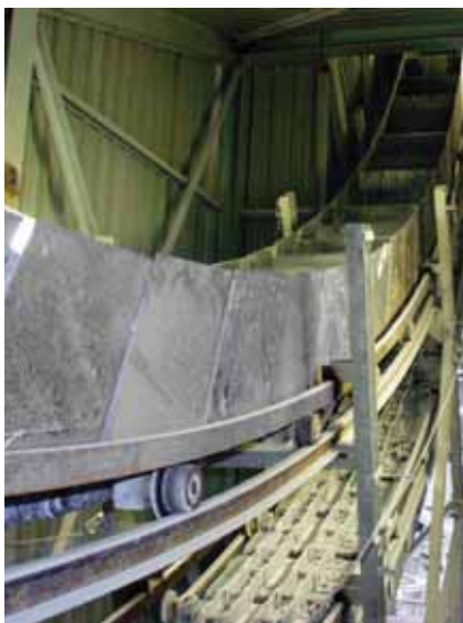
Box conveyors generally used for conveying material with inclination above 40°.
