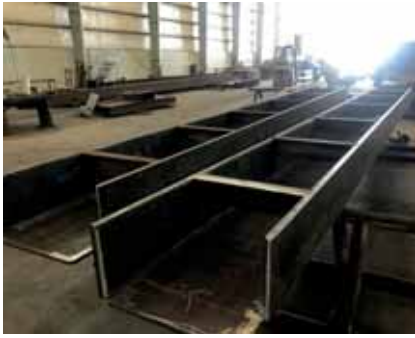
UBT engineering at work, digging leg fabrication for barge unloader.
