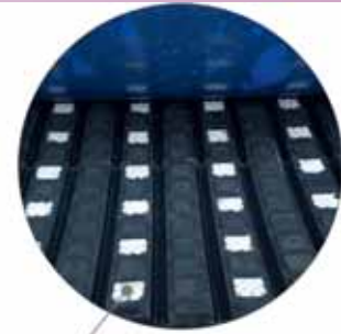
Abrasion-resistant tiles fully enclosed by rubber.
