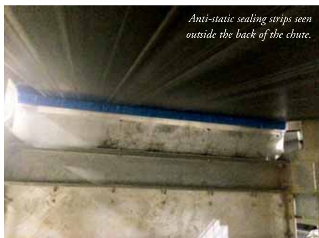
Anti-static sealing strips on the inside of the chute.
