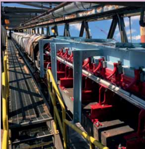
AFTER: ASGCO® Slide-N-Roll® system along with new engineered chute design and proper load zone support with sealing rubber.
