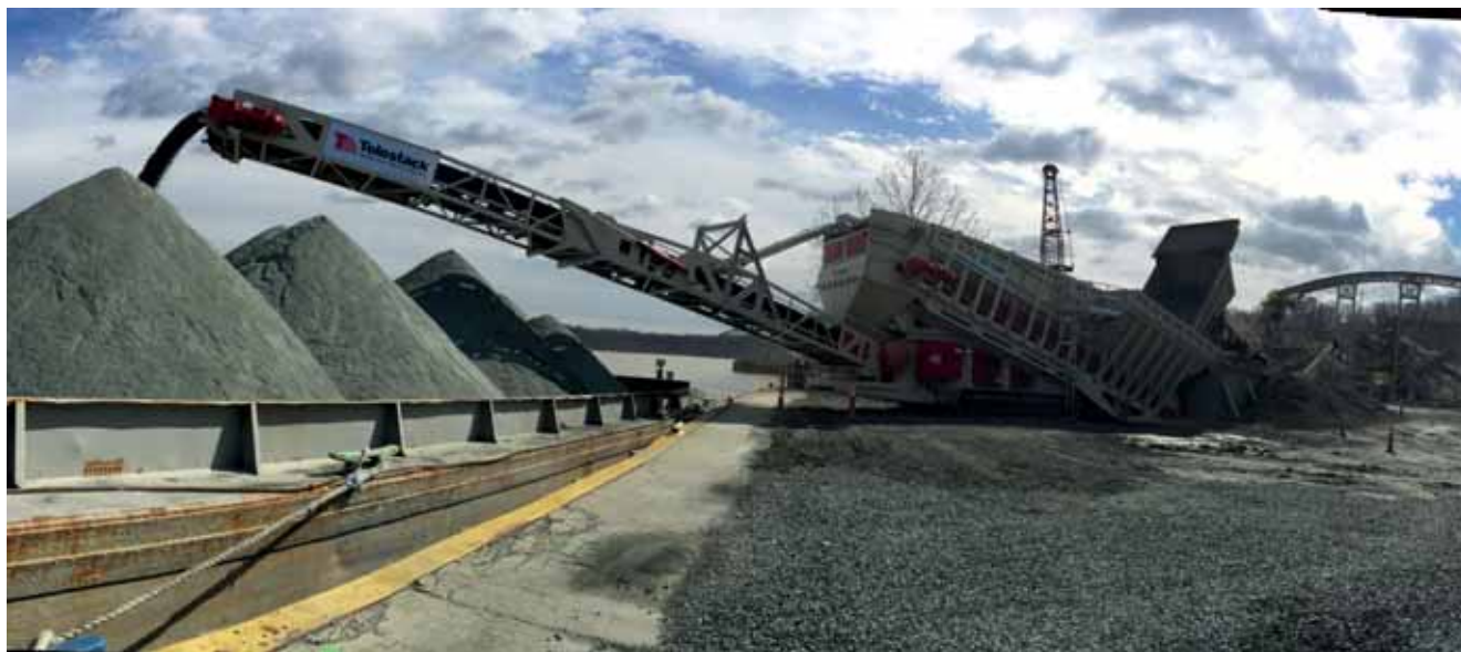
Weighing 120 tonnes in weight, 35 metres in length and 8 metres in height, the Telestack TITAN T-1600-8 is the largest truck unloader in the international market. With a throughput in the region of 2,000tph, this unit is loading barges in North America.
