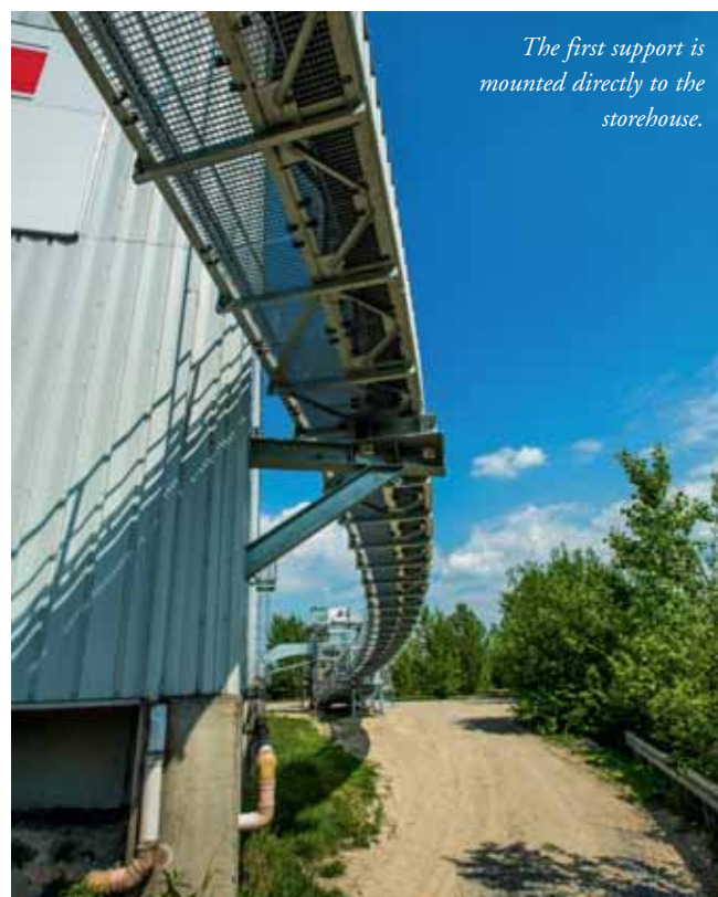
The inclination of the pipe conveyor measures 18.6° at the point shown.
