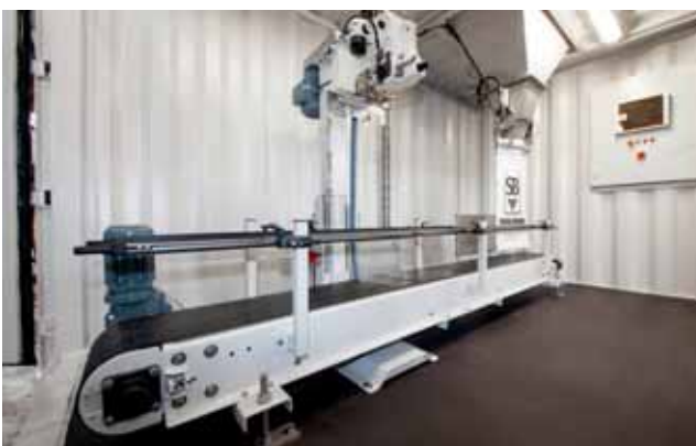
Bag filling line with operator panel in bottom container.
