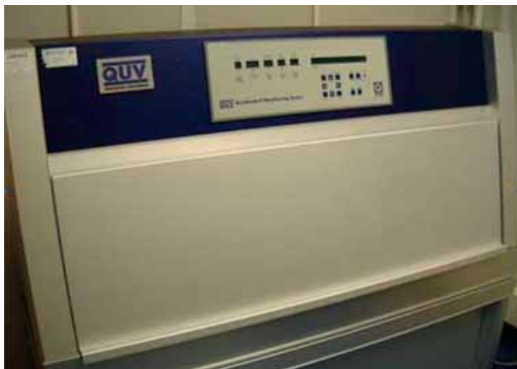
Figure b: Laboratory testing equipment used to simulate weathering exposure. Image © IBE-BVI Group
