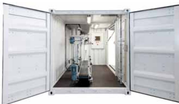
Bag filling spout with transport conveyor and sewing machine.
