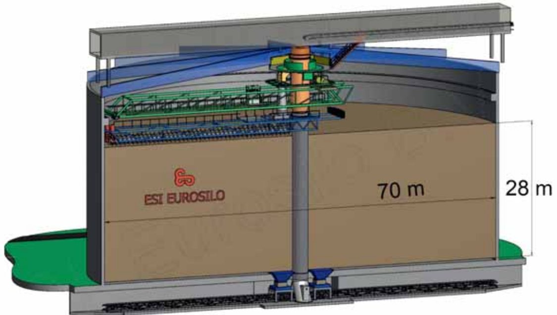
Fig 6: Typical layout of a Eurosilos for storing (wood) pellets
