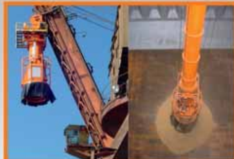
Dust trap - Upgrading
