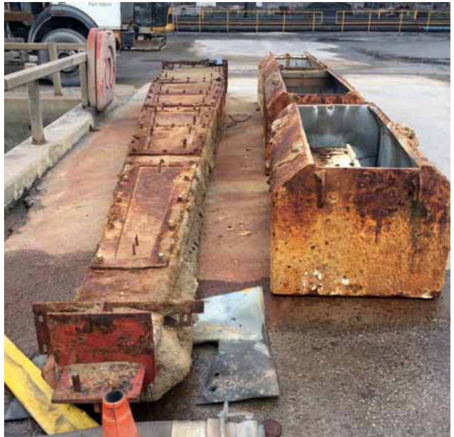
Without Kingfisher's wear-resistant liners, slag granulation equipment can quickly become damaged and, eventually, unusable.
