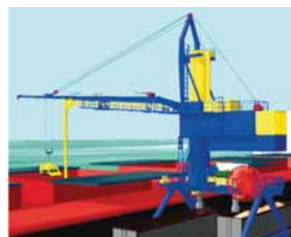
Figure 5: Maximum load-bearing capacity of the winch (3.5t) requires several smaller bucket loaders.
