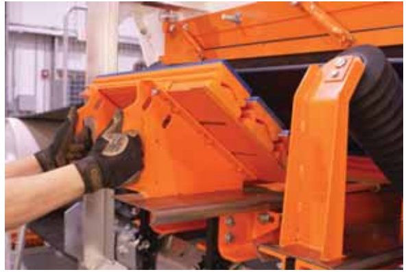
Designed for ease of service, modular components allow faster, safer changeouts by one person.
