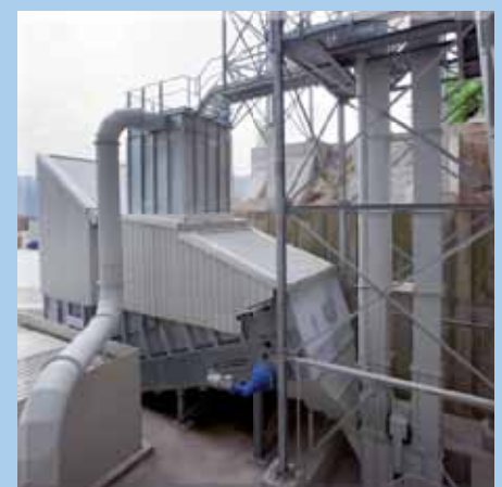
"TIREX"- Receiver from trucks and feeder for several bulk materials
