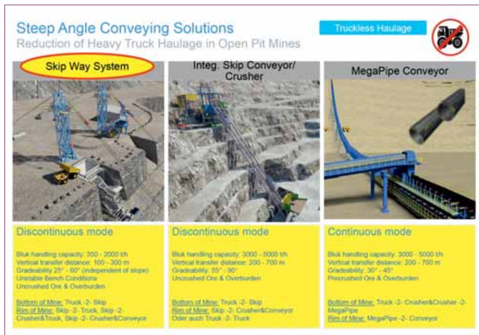
Fig. 17: Reduction of heavy haul traffic in open-pit mines through use of steep-angle conveying systems.
