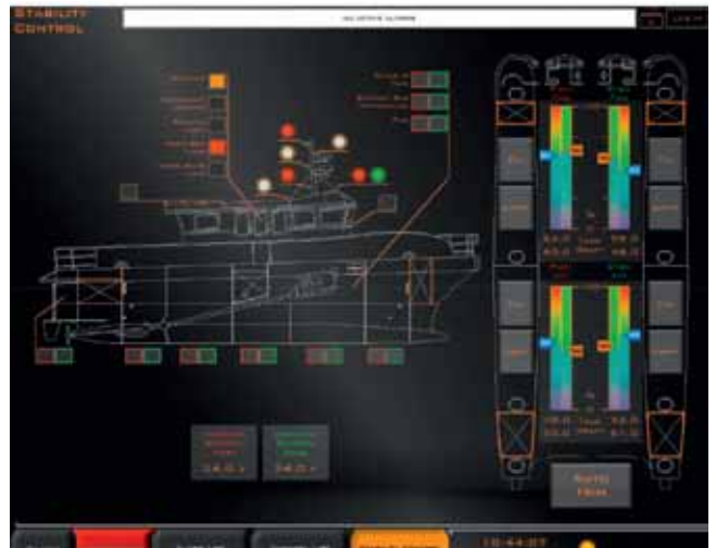
Ship trim and draught conditions can be easily evaluated and optimized using Servowatch's new ServoTrim system
