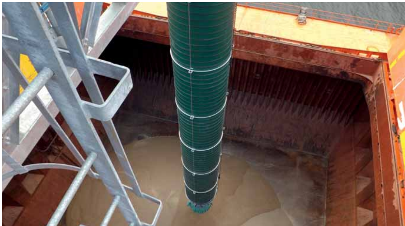
Cleveland Cascades shiploader handling biomass pellets at rates of up to 2,000 tonnes per hour in Prince Rupert, BC, Canada.
