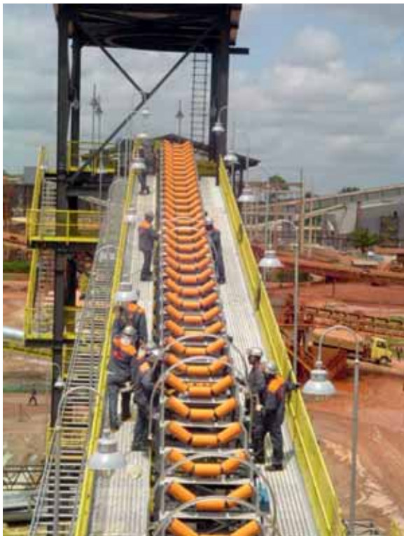
Left: Alumina conveyor 1,500tph. Above: VALE Carajás, Brazil: classification tower and conveyors.
