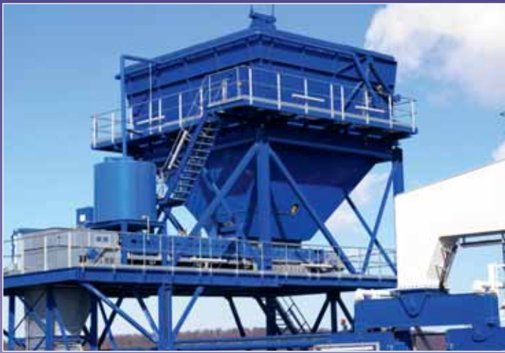
Hopper cars for ship unloading
