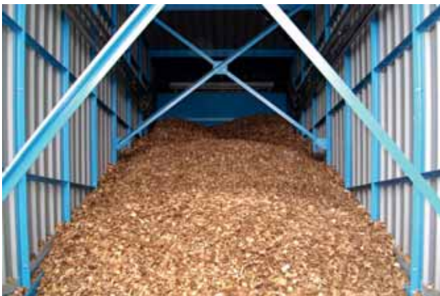
The Samson™ handles wood chips from walking floor trucks for intake to a biomass boiler for plant steam generation at two famous brewery complexes (©AUMUND).
