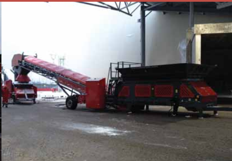
Mobile Hopper feeder fed from wheel loader in warehouse
