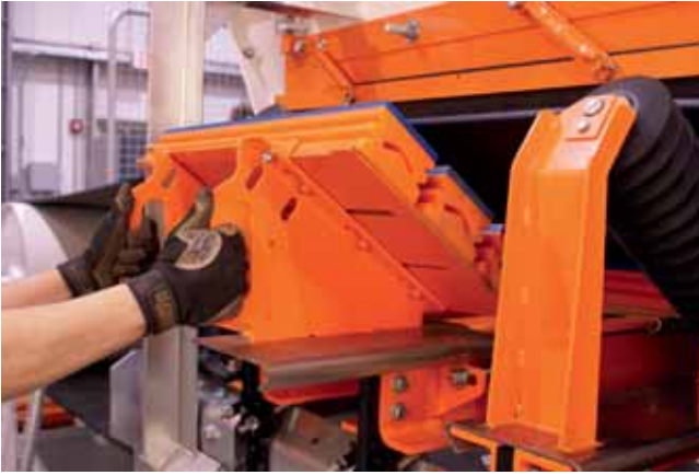
Modular components such as track-mounted pulleys and cradles can deliver slide-in / slide-out convenience.
