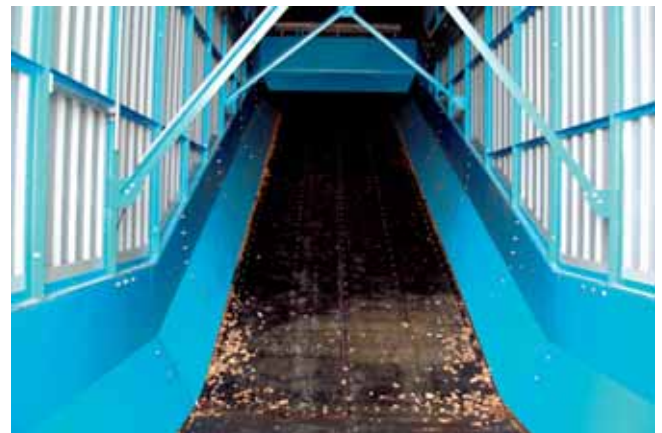
The Samson™ handles wood chips from walking floor trucks for intake to a biomass boiler for plant steam generation at two famous brewery complexes (©AUMUND).
