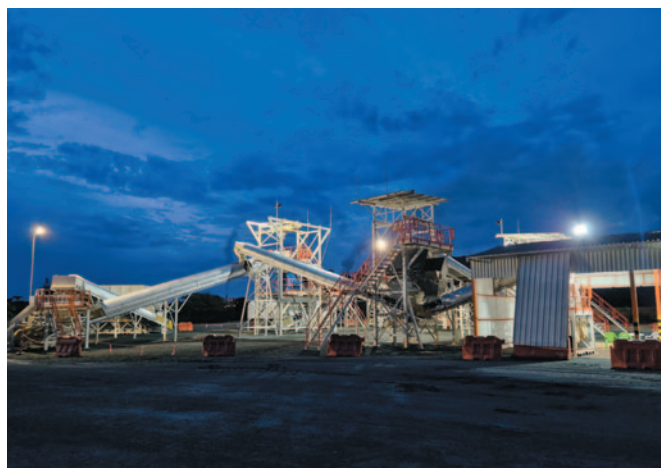
De Regt Conveyor Systems designed, manufactured and assembled a complete tailor-made installation in South America, consisting of a receiving hopper, multiple conveyor systems and a crusher.
