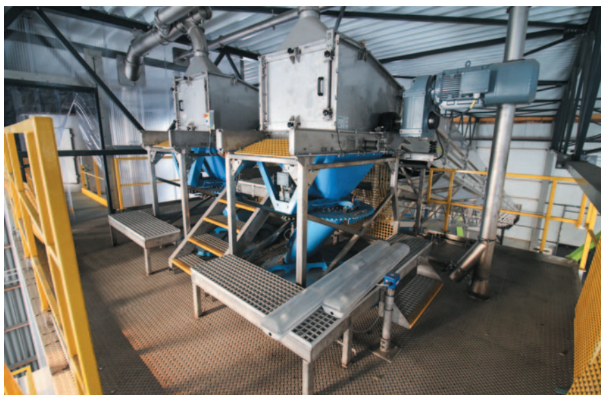
For a customer specialized in fertilizer processing, De Regt Conveyor Systems supplied a complete bagging installation for filling both big bags and 20kg packaging units.
