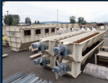
CONTINENTAL LIVE BOTTOM DUAL SCREW ENCLOSED METERING BINS
