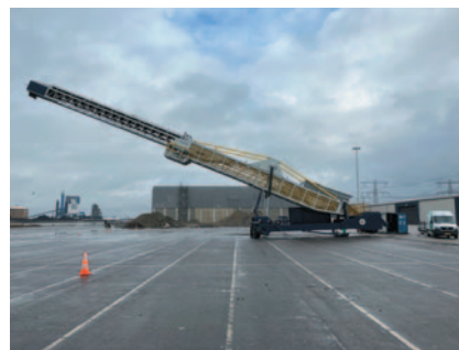
Mobile telescopic conveyors are ideally suited for loading and unloading vessels or filling storage warehouses.
