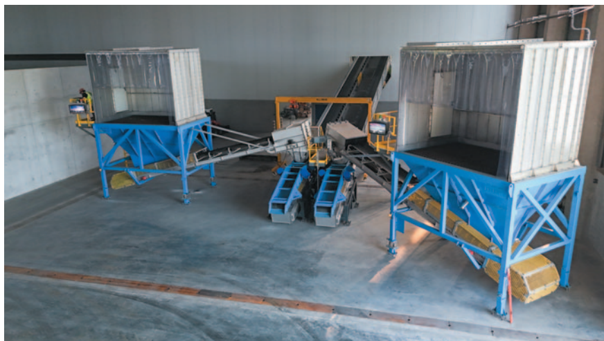
For a customer specialized in fertilizer processing, De Regt Conveyor Systems supplied a complete bagging installation for filling both big bags and 20kg packaging units.
