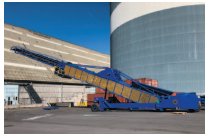
Mobile telescopic conveyors are ideally suited for loading and unloading vessels or filling storage warehouses.
