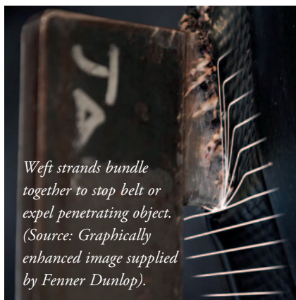
Tested to destruction — more than 500% superior longitudinal rip resistance and up to 300% greater impact resistance compared to conventional belting.
