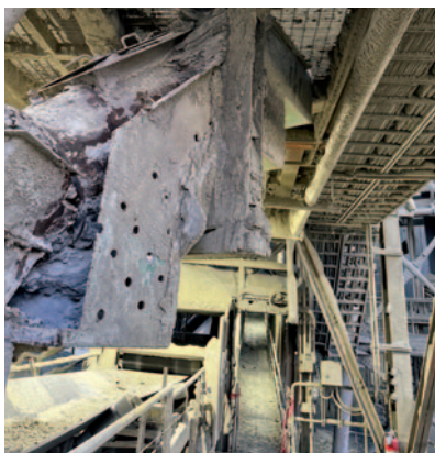
The problem: A misaligned step chute at a cement facility was leading to off-centre loading and spillage.
