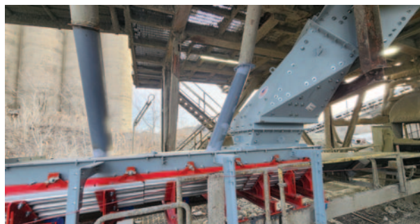
The solution: ASGCO used point cloud scanning and 3DEM simulation to identify the issue and engineered a custom center-loading chute w/ modern skirting.
