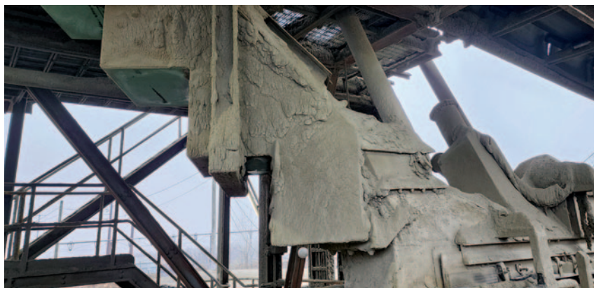
The problem: A misaligned step chute at a cement facility was leading to off-centre loading and spillage.
