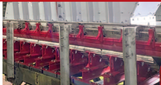
ENGINEERED LOAD ZONES & IMPACT BEDS
