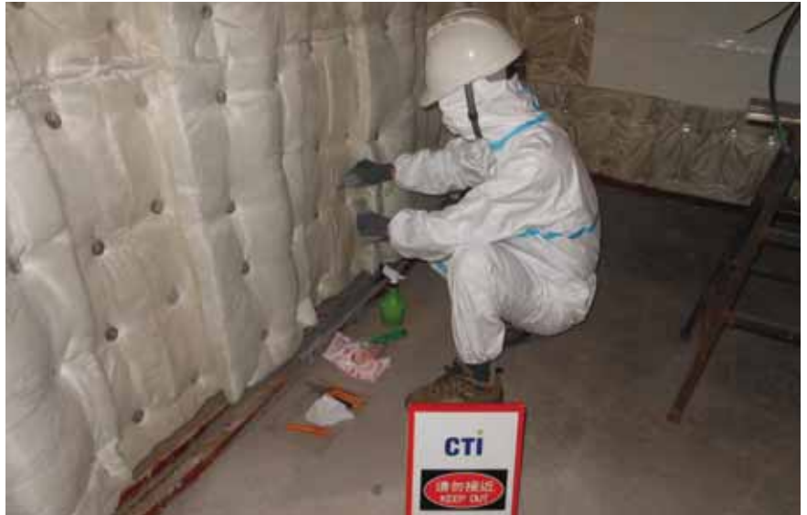
A CTI technician collecting asbestos (above) and hazardous material (below) samples.
