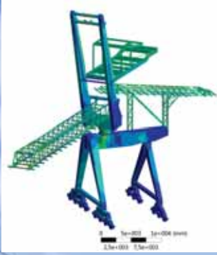
Slewing boom shiploader and FEM — Finite Element Analysis (TMSA, Brazil).
