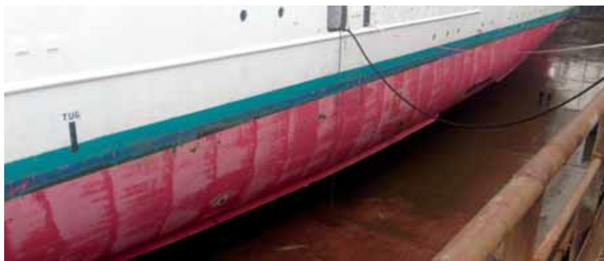
Low-friction self-polishing antifouling paints have excellent performance after years of service.
