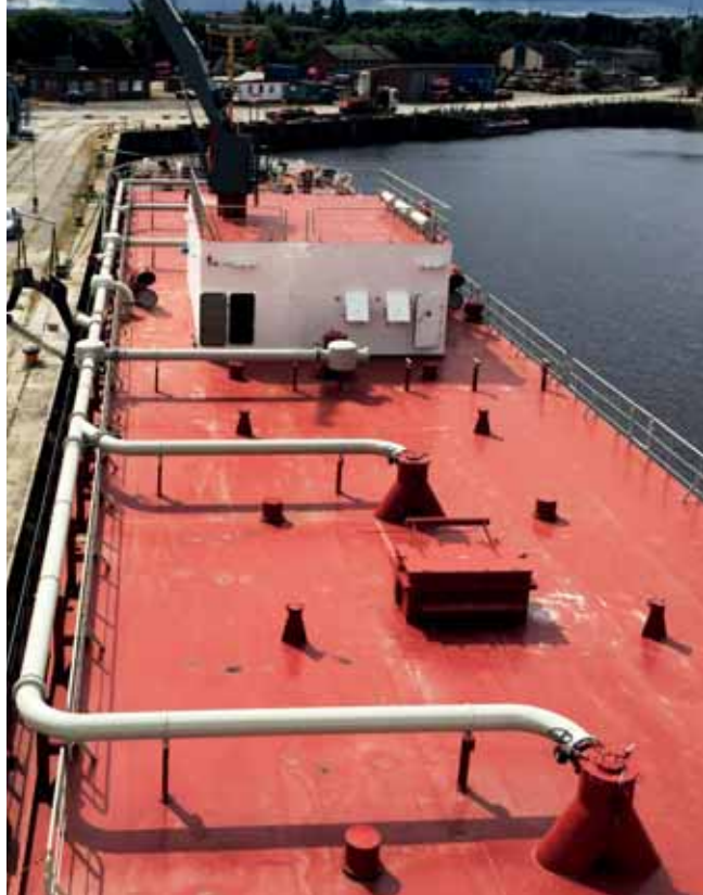
Fig. 6: Cement distribution to the holds.
