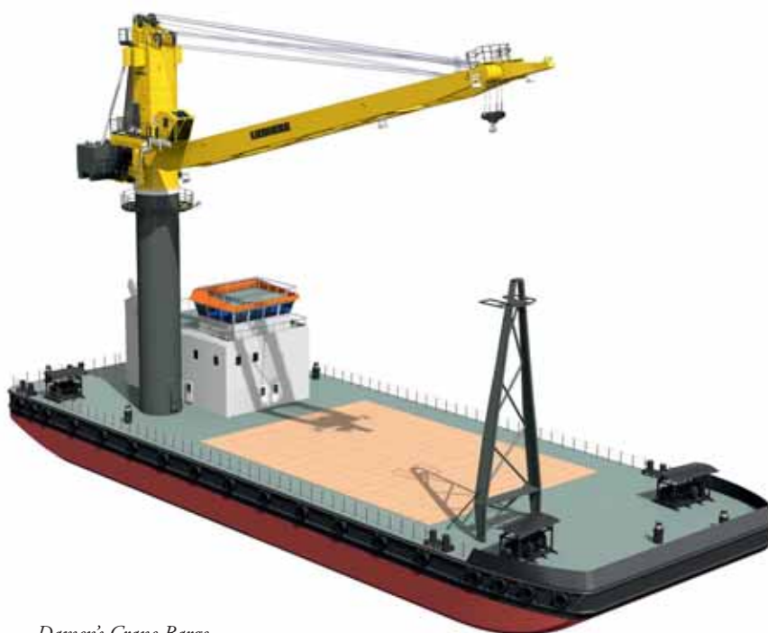
Damen's Crane Barge 6324 is a low-cost transshipment barge designed for ship-to-ship, ship-to-barge or ship-to-quay operations.
