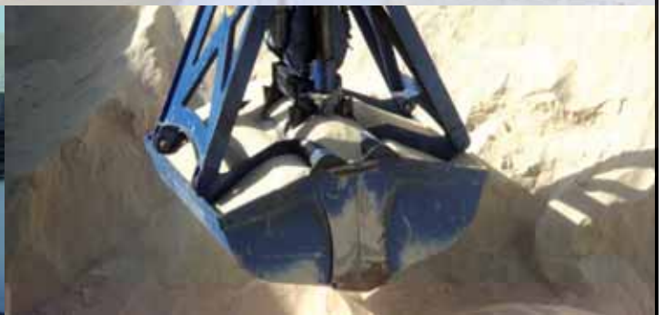
Mechanical one rope clamshell bucket with remote control
