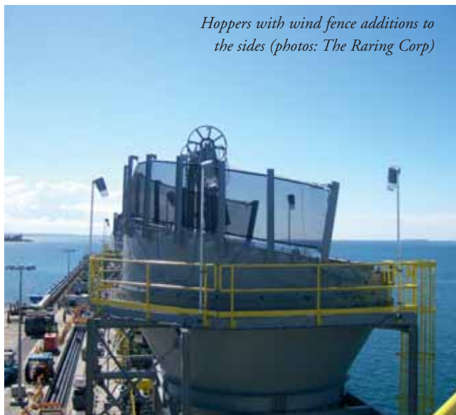
Unloading hopper dust control.
