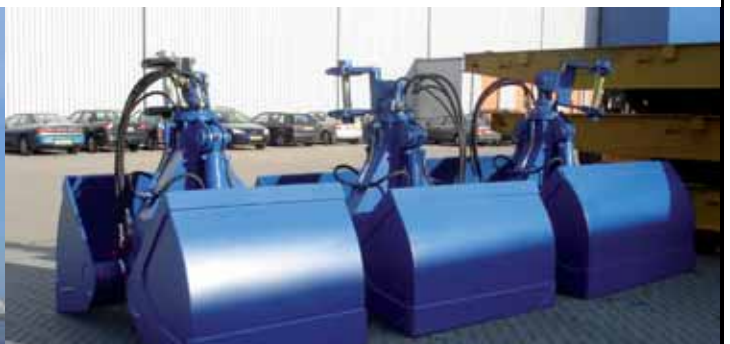
Hydraulic clamshell bucket with connection piece
