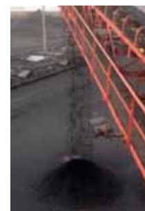
Coal treated with approximately 20 gram Freko Foam A per tonne.
