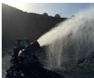
Spraying of Freko Crust with fogging unit.
