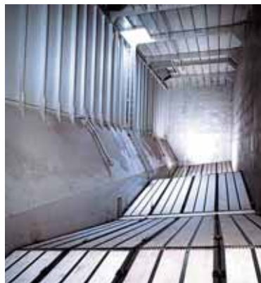
The revolutionary IBAU HAMBURG Tunnel concept: Midship tunnel with the IBAU Pump and aeration panels.
