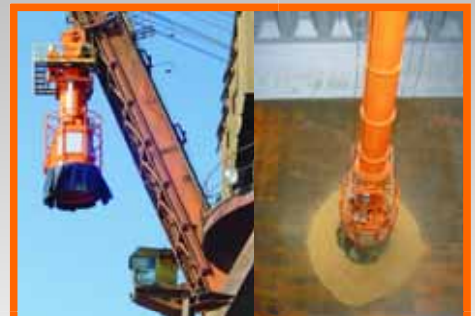
Dust trap - Upgrading
