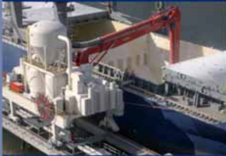
Rail Mounted Ship Unloader
