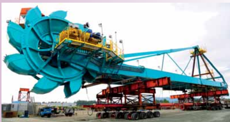
Fig. 2. The 7,000tph (coal), stacker/reclaimer pictured here, also designed and supplied by EMS-Tech Inc., highlights the enormous Boom Head End section being prepared for transfer to the barge that will deliver the large assembled units to Neptune Coal Terminals, in North Vancouver where it will be final assembled and commissioned.
