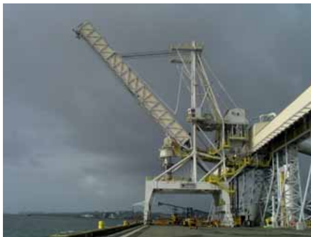
AGP — Aberdeen/WA/USA: 1,500tph grains, with a shuttle conveyor along the berth, feeding the loader and gaining important extra useful length of the pier (TMSA Brazil).
