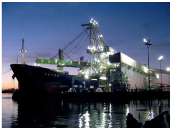
AGP — Aberdeen/WA/USA: 1,500tph grains, with a shuttle conveyor along the berth, feeding the loader and gaining important extra useful length of the pier (TMSA Brazil).
