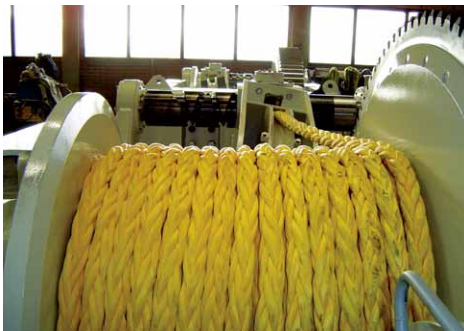
Lankhorst mooring rope on mooring winch.
