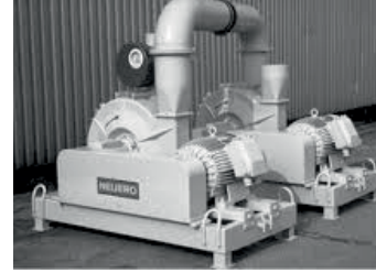
Fan with Air Flow Regulator (1960)
