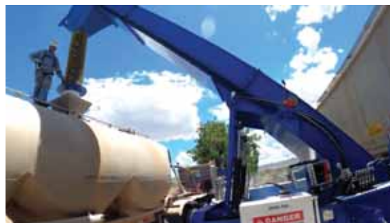
Cambelt's Scorpion™ line of transloading conveyors are designed for situations where it is impractical to have a fixed conveying system.
