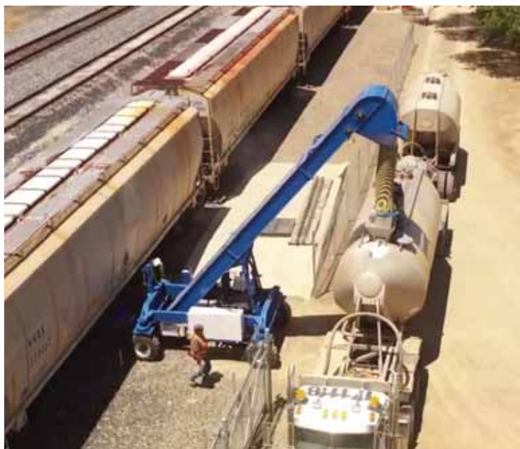
Cambelt's Scorpion™ line of transloading conveyors are designed for situations where it is impractical to have a fixed conveying system.
