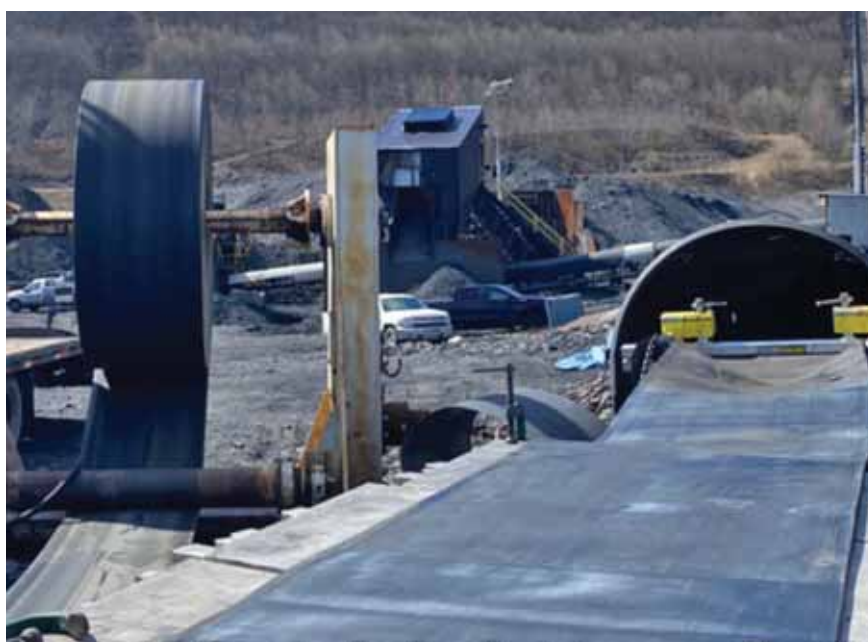
Picture of a completed "Seam-less" splice after being removed from the vulcanizing press during and overland belt installation.
