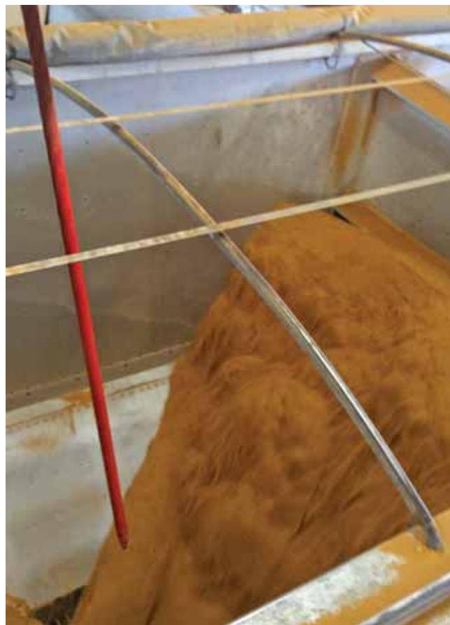
The operator uses remote controlled hydraulics to drive the probe down and loosen hardened meal in a hopper railcar (left) or truck trailer (right).
