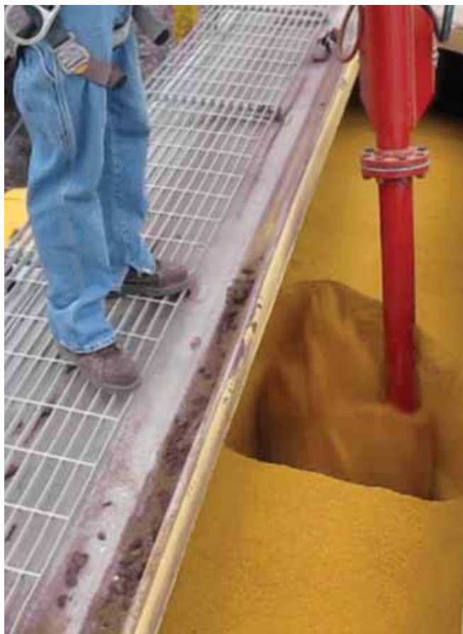
The operator uses remote controlled hydraulics to drive the probe down and loosen hardened meal in a hopper railcar (left) or truck trailer (right).
