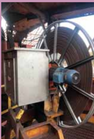
Monospiral reel for reeling length up to 370m
