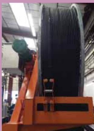
Small level wind reel with guiding device (TRV) for reeling length from 300m up to 800m.
