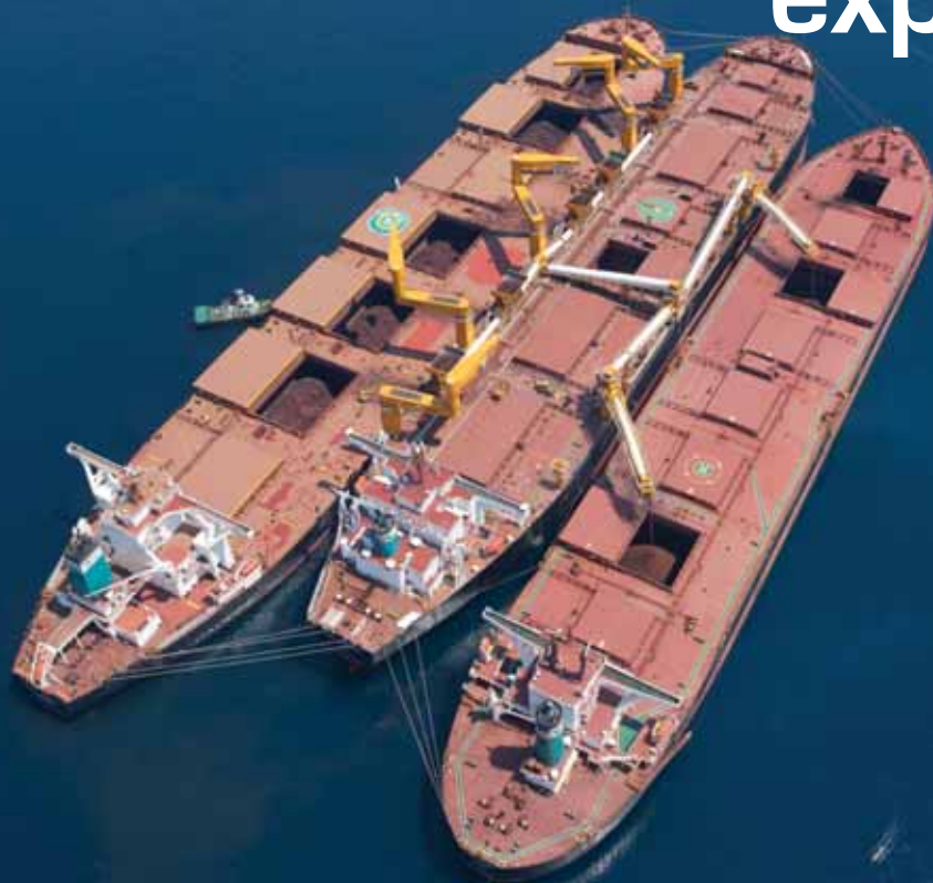
The Ore Sossego transshipper in operation.
