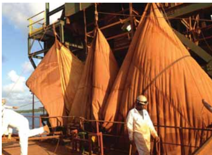
Old technology (left): dust curtains manually installed around a bauxite shiploader hatch in the Caribbean (Jamaica). New technology (below) — a completed enclosed, long distance pipe conveyor handling petcoke and sulphur (Venezuela).
