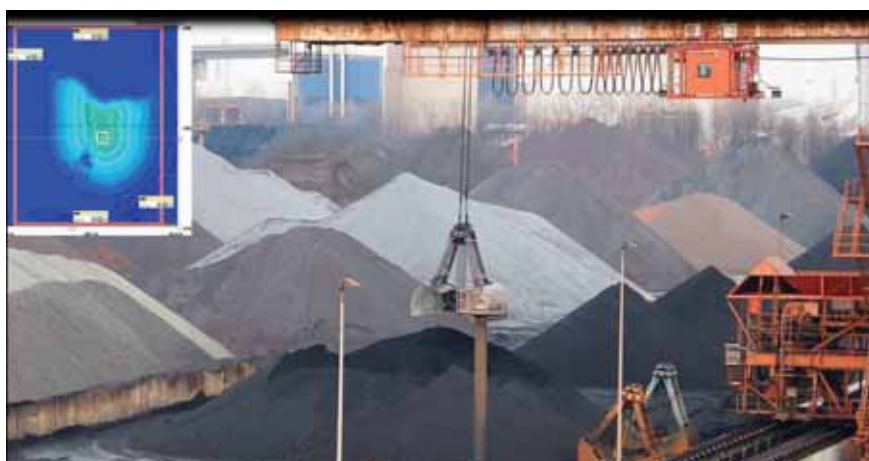
Grab 3D live tracking, bulk material scan of backreach area.
