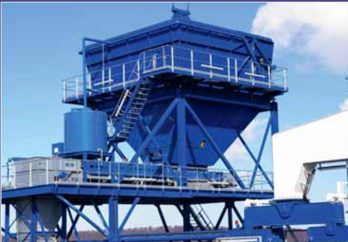
Hopper cars for ship unloading
