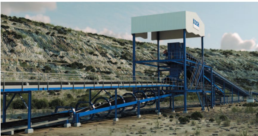
KOCH's TrackBelt system is specifically developed for long-distance bulk material transport, starting from conveyor lengths of approximately 500m and extending up to 40km in a single continuous loop.
