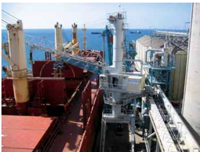
This unloader was supplied in 1993, for a rate of 190tph. In 2008, Neuero upgraded the 25m boom, increasing capacity to 250tph, and lengthening the horizontal boom length by 10%.
