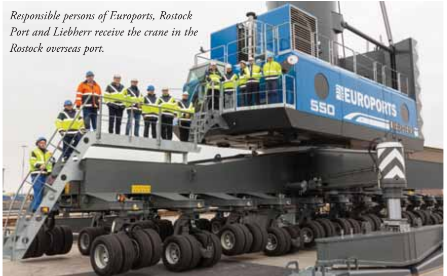
With a tower height of over 30 metres and a jib length of 54 metres, the new Liebherr LHM 550 Mobile Harbour Crane is the largest at the Euroports Terminal.
