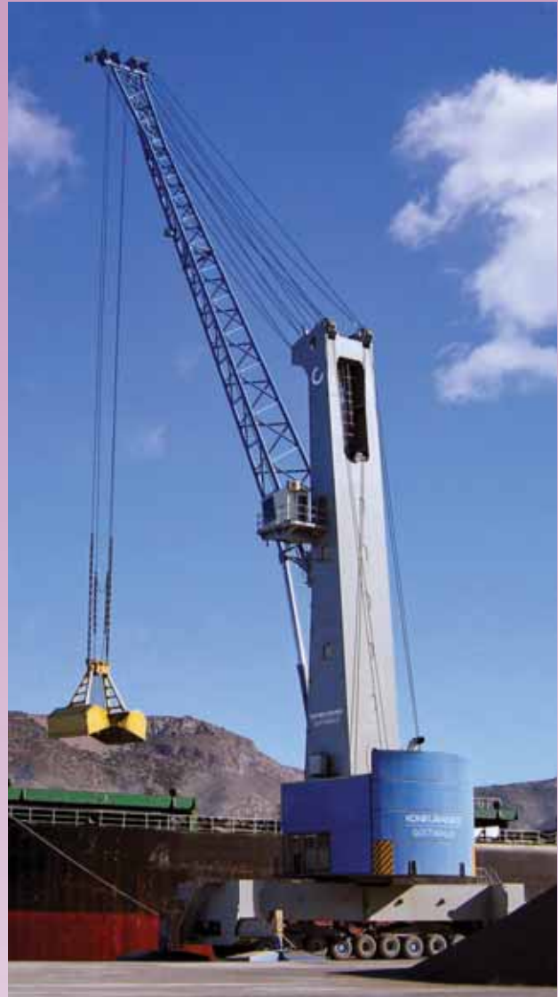
Konecranes Gottwald Model 8 mobile harbour cranes are in high demand around the globe. In 2019, three will be delivered to the United Arab Emirates where they will handle predominantly inbound as well as outbound bulk material. The picture shows a similar crane handling coal.
