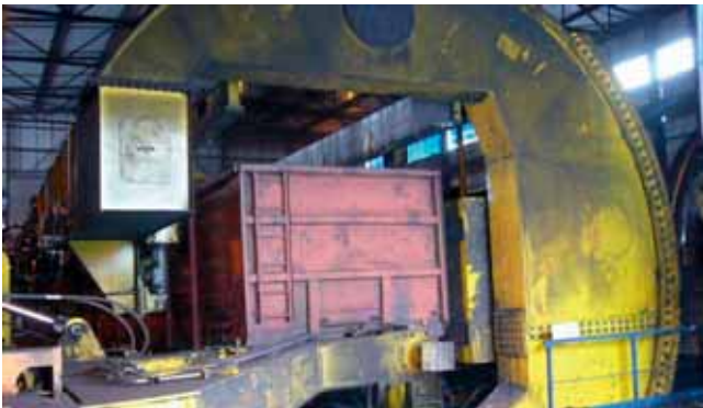
Pic. 3 TK's tandem rail car dumpers operating at Ust Luga Coal Terminal since 2005.
