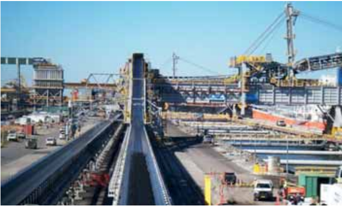
ContiTech has supported the expansion of the Newcastle Coal Infrastructure Group's coal export terminal with several kilometres of steel cord belting. (Photo: ContiTech)
