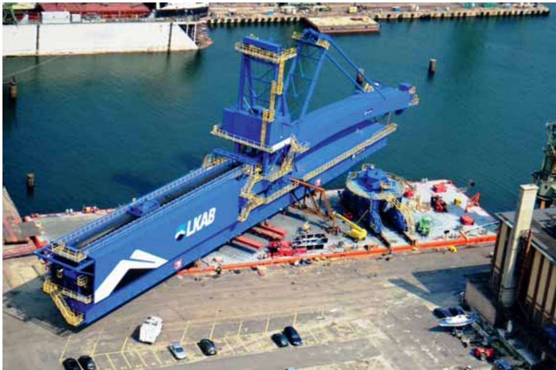
Pic. 5.1 The fully assembled shiploader going on board for departure.
