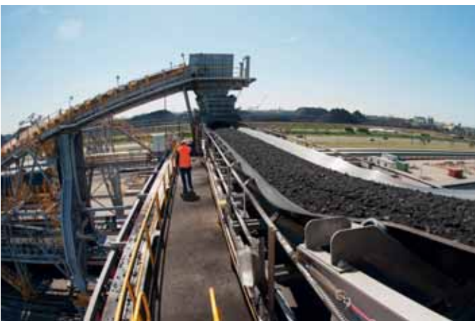
The supplied steel cord belts also include energy-optimized conveyor belts. Thanks to special rubber compound, energy consumption during transport can be lowered by up to 25%, allowing a reduction of energy costs and CO 2 emissions overall. (Photo: ContiTech)
