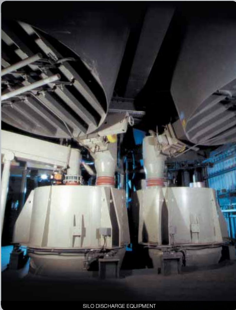
SILO DISCHARGE EQUIPMENT
